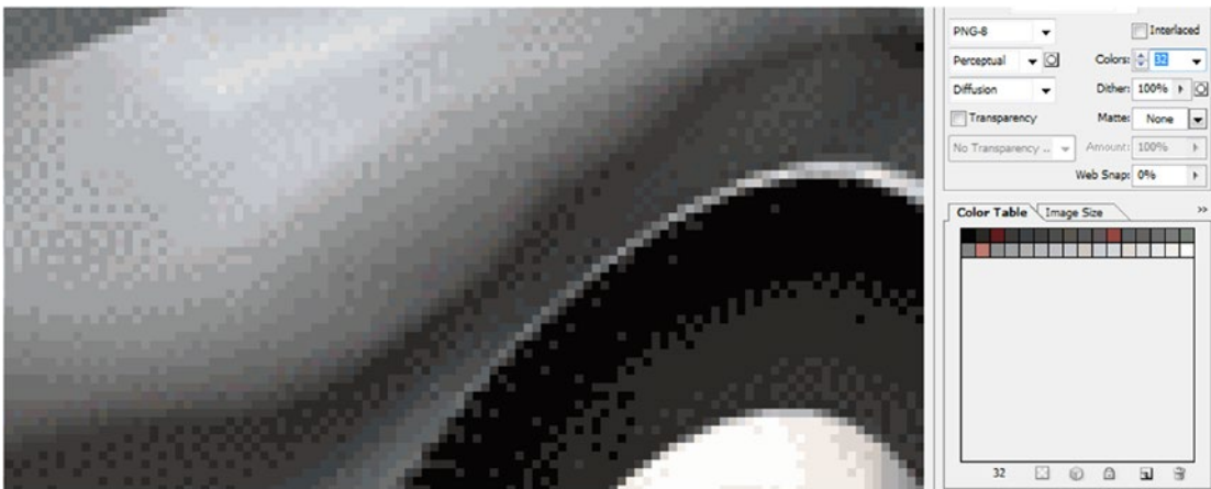
Figure 2-5. Setting dithering to the Diffusion algorithm and 32 colors (5-bit color) with 100 percent dithering for PNG5 output
