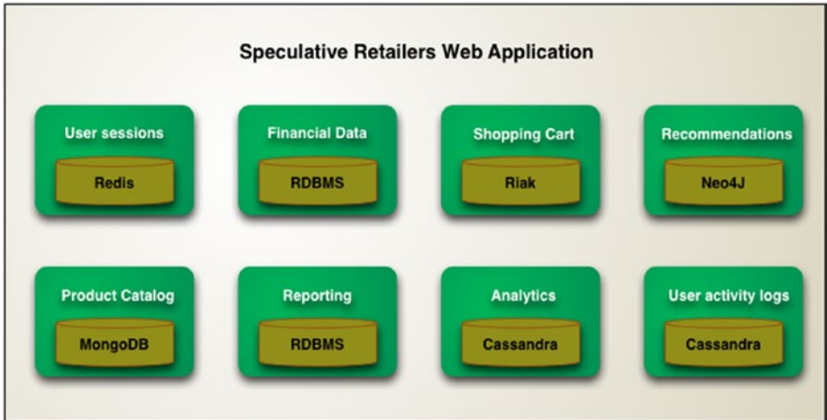
Figure 7-1. Polyglot persistence example (source: Martin Fowler)
