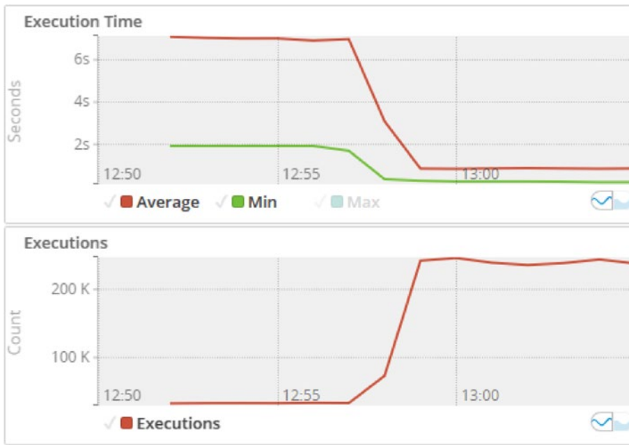
Figure 14-1. The query metrics before and after the index was added
