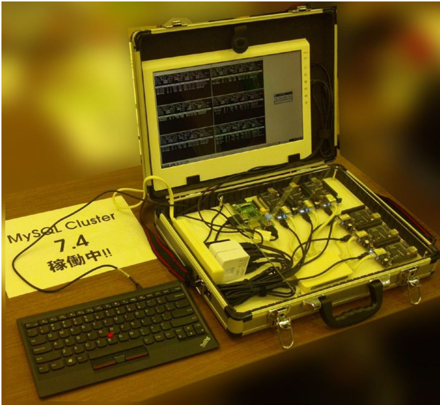
Figure 3-4. NDB Cluster running on single board computers
