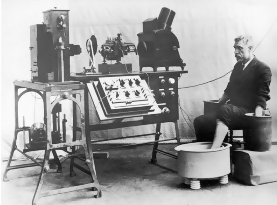
Figure 12-1. An early electrocardiograph from 1911. Note the arms and one leg of the patient immersed in buckets, which contain a saline solution to conduct the body's current. Modern ECG sensors are still based on this three-point principle, but optical sensors rely on a completely different physical process to measure heart rate.
