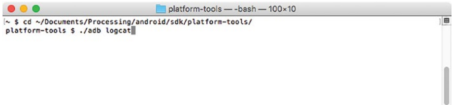
Figure 3-2. Terminal session on Mac displaying the commands to run logcat
