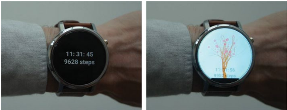
Figure 12-11. Final version of the tree watch face, in ambient (left) and interactive (right) modes
