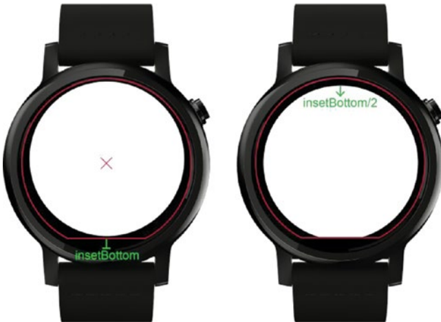
Figure 10-9. “Chin” in a Moto 360 smartwatch. Graphics centered at the screen center (left), and translated by half of the bottom inset to properly center them with respect to the bezels
