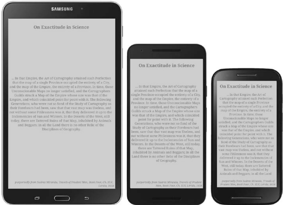
Figure 4-23. From left to right, text output on a Samsung Galaxy Tab 4 (7", 1280 × 800 px, 216 dpi), Nexus 5X (5.2", 1920 × 800 px, 424 dpi), and a Moto E (4.3", 960 × 540 px, 256 dpi)
