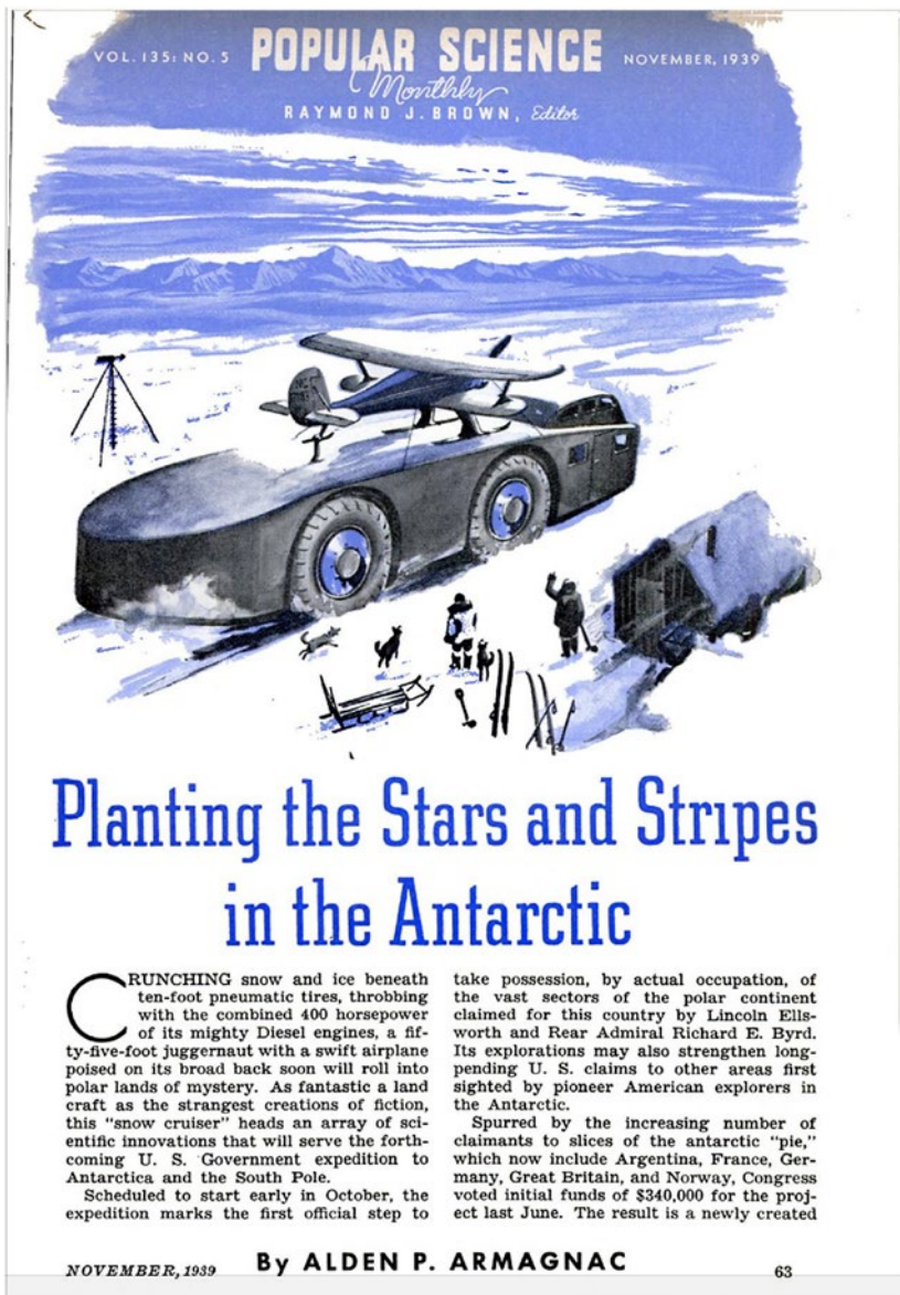
Figure 16-1. Antarctic Snow Cruiser. A hybrid tractor, tank, laboratory, and aircraft carrier for Antarctic exploration intended for use by Admiral Byrd in 1939. Alas, its weight was too much for the snow surface, and it was never used. Popular Science Monthly , v. 135, no. 5, Nov., 1939. http://bit.ly/2eJOofM : public domain.
