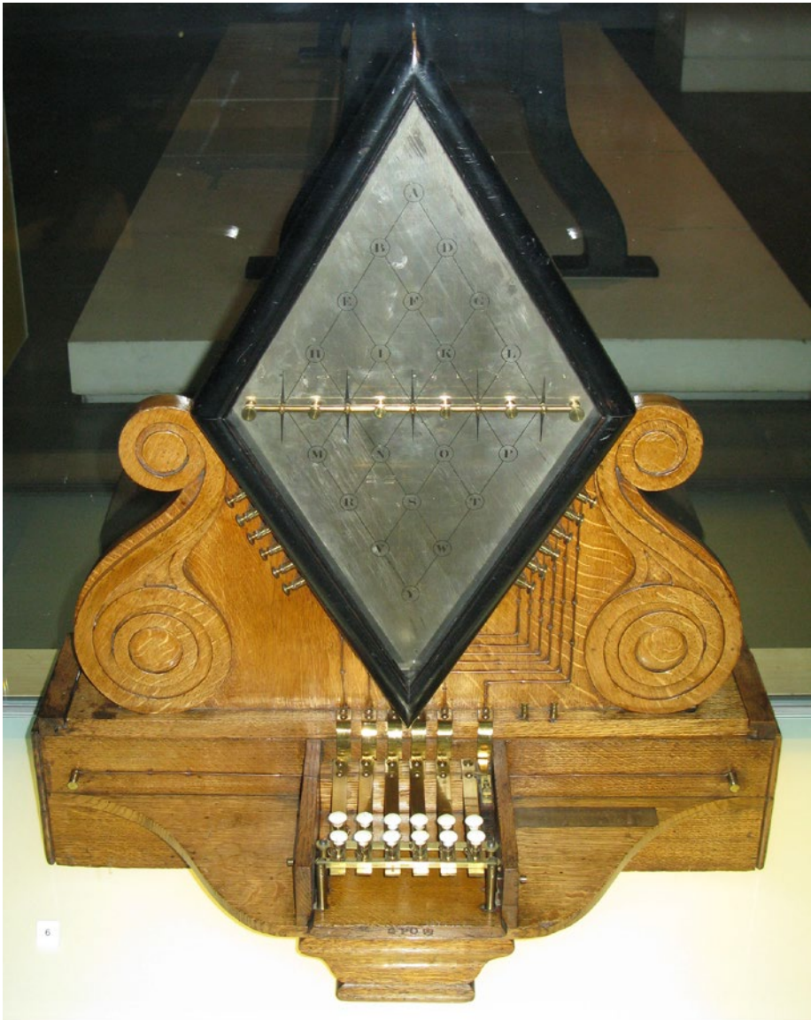
Figure 7-3. Five-needle electric telegraph invented by Charles Wheatstone (of the Wheatstone bridge), 1837. The telegraph was used to signal when trains arrived and left stations. Now at the London Science Museum. Photo by Wikipedia user Geni; license CC-BY-SA GFDL.
