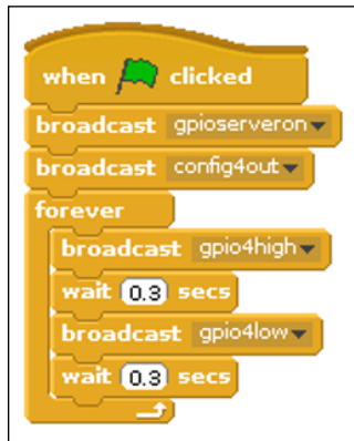
FIGURE 16-7: Scratch program to blink the LED.
