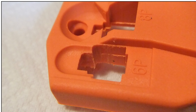
Figure 15-5: Crimp tool modification.
