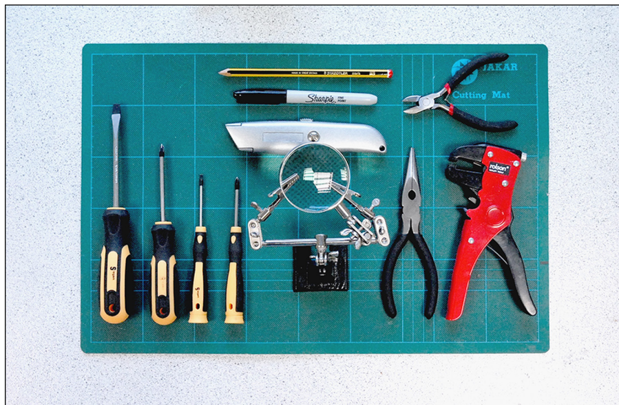
Figure 2-4: Some essential light fabri- cation tools.
