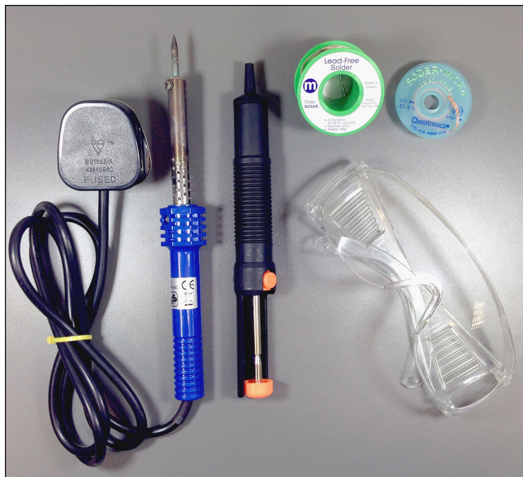
Figure 2-3: An entry-level soldering iron and essential accessories.
