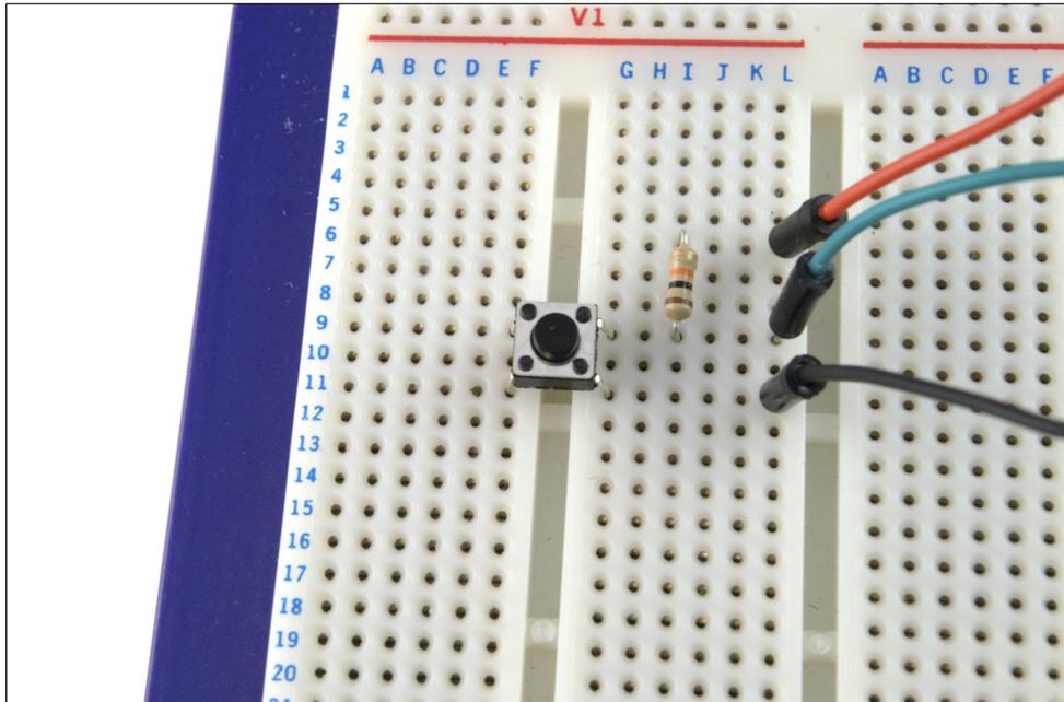
FIGURE 12-7: A sample breadboard circuit, with loose-fitting components
