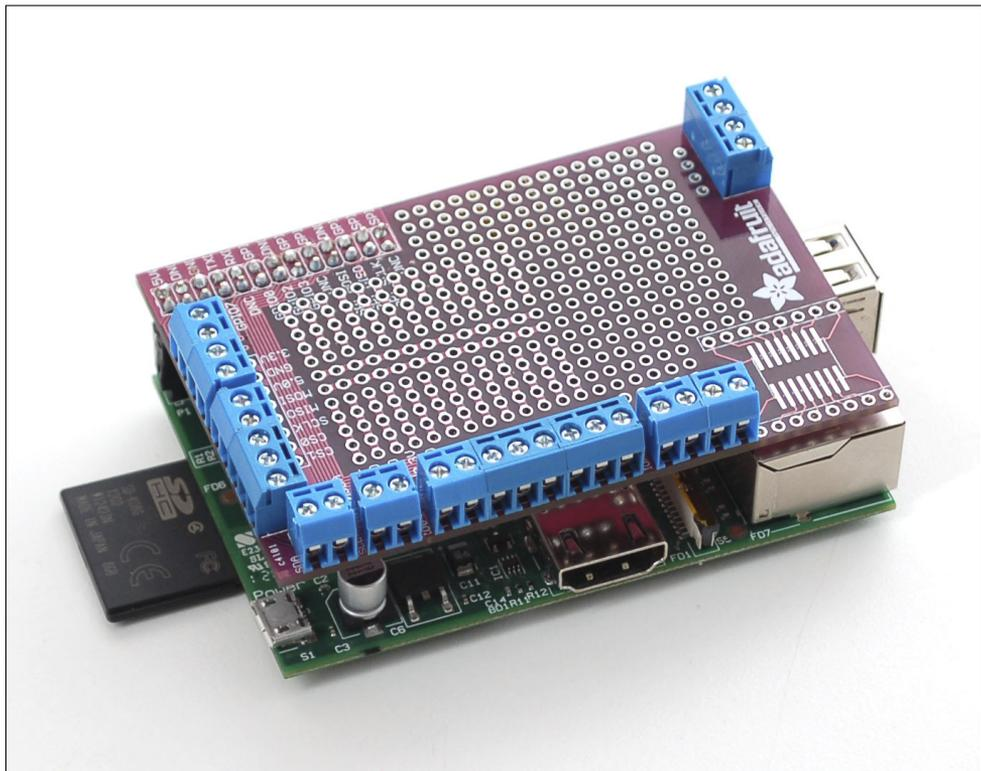
The design and layout of the Prototyping Pi Plate will be familiar to anyone who has used an Arduino microcontroller. An add-on board with the same footprint as the target device, designed to connect to on-board headers and sit above the surface of the original board is a common sight in the Arduino world, where such add-on boards are known as *shields*. The idea for the Prototyping Pi Plate, in fact, comes from Adafruit's self-designed Protoshield add-on for the Arduino.
