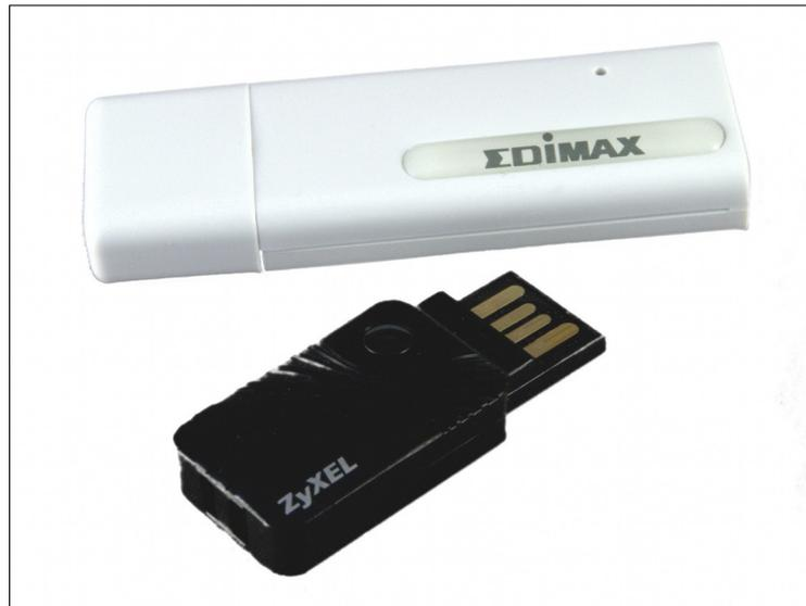
FIGURE 1-8: Two USB wireless adapters, suitable for use with the Raspberry Pi
