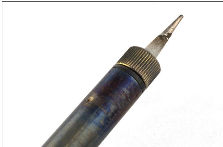
**FIGURE 12-10:** A soldering iron tip that is in the process of being tinned with solder
