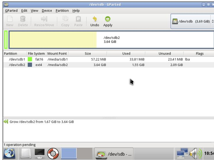
FIGURE 5-8: Parted Magic's Partition Editor tool, after resizing the partition
