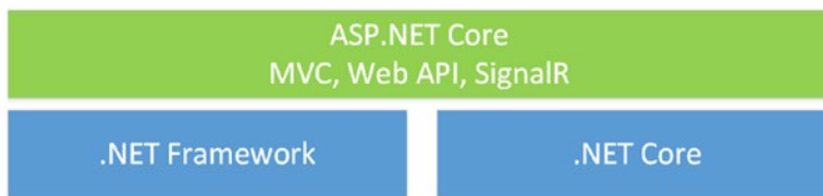
Figure 2-2. Compatibility of ASP.NET Core with .NET Framework and .NET Core
