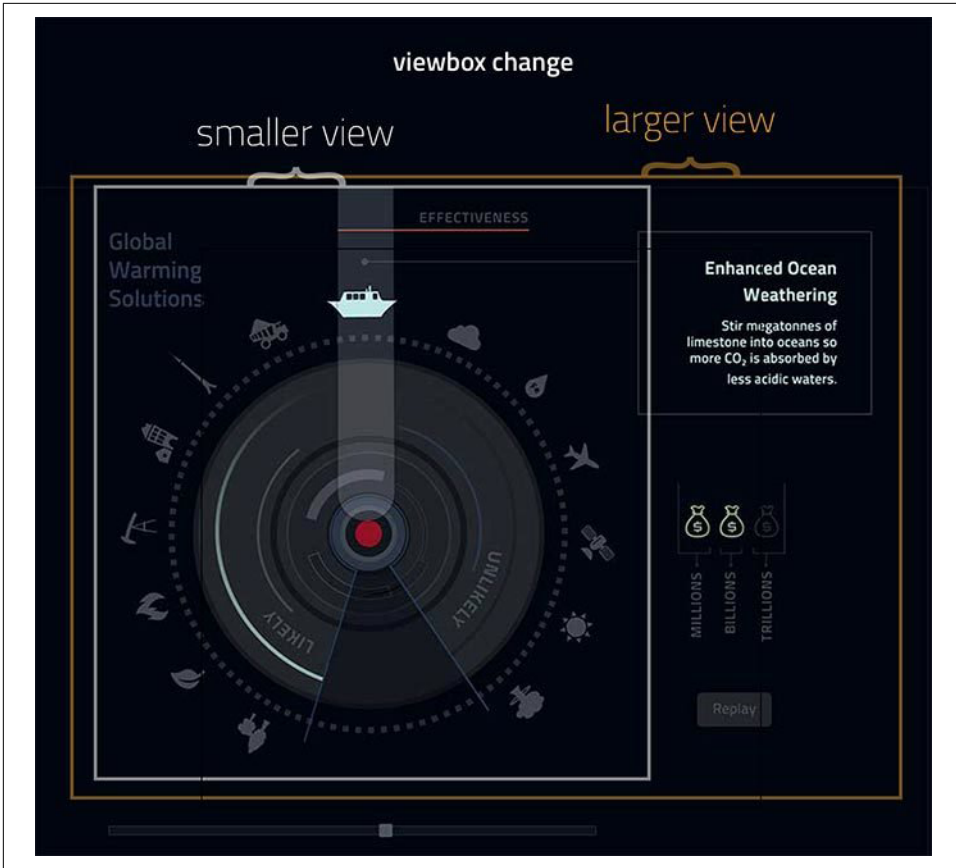
Figure 16-5. The viewBox shifts for mobile and desktop views of the infographic
