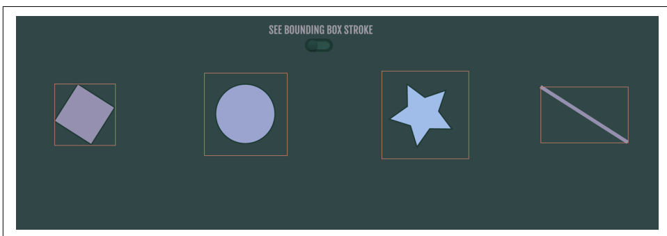
Figure 15-8. When an SVG element is transformed, the bounding box doesn't go with it —there are no diagonals; the box expands and creates a rectangle, even with circles and lines
