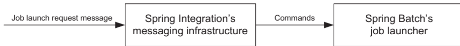
Figure 11.7 The Spring Integration quick-start uses Spring Integration messages to trigger Spring Batch jobs.
