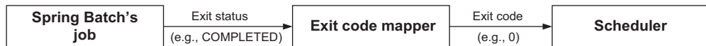
Figure 4.6 The command-line job runner uses an exit code mapper to translate the string exit status of a Spring Batch job into an integer system exit code. The triggering system—a system scheduler here—can then use this system exit code to decide what to do next.
