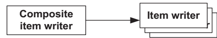
Figure 6.11 A composite item writer delegates writing to a list of item writers. Use this pattern to send items to several targets, like a database and a file.
