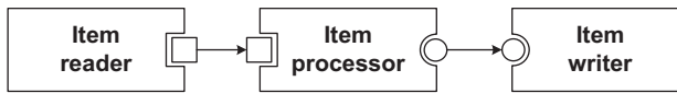
Figure 7.3 The item processor of a chunk-oriented step can produce objects of a different type (represented by circles) than the read items (squares). The item writer then receives and handles these new objects.
