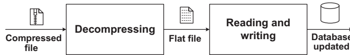
Figure 1.6 The Spring Batch job consists of the following steps: decompression and read-write.
