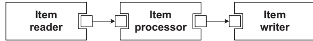
Figure 7.2 In the processing phase of a chunk-oriented step, you can choose to only change the state of read items. In this case, the item reader, processor, and writer all use the same type of object (illustrated by the small squares).
