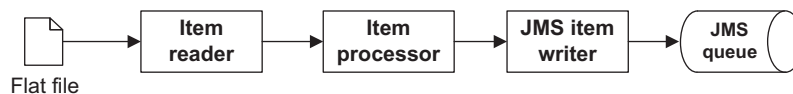
Figure 6.9 An application puts messages on a JMS queue with a JMS item writer. Applications often use JMS to communicate with each other in a decoupled and asynchronous way.
