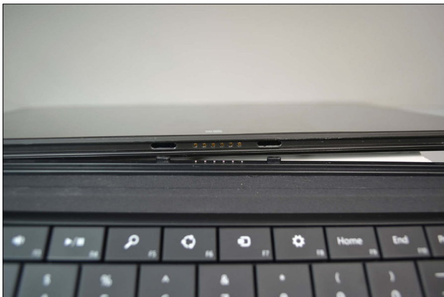
Figure 2-7: Match the Touch or Type Cover keyboard's connector with the connector on the bottom of your Surface, and they click into place.
