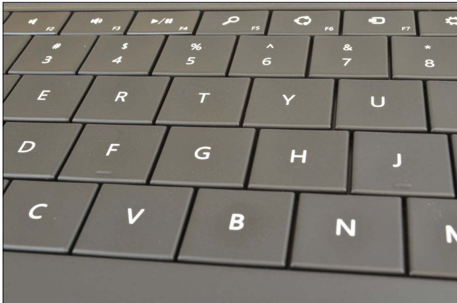
Figure 5-2: The Surface Type Cover and Type Cover 2 keyboards offer mechanical keys that move when touched.
