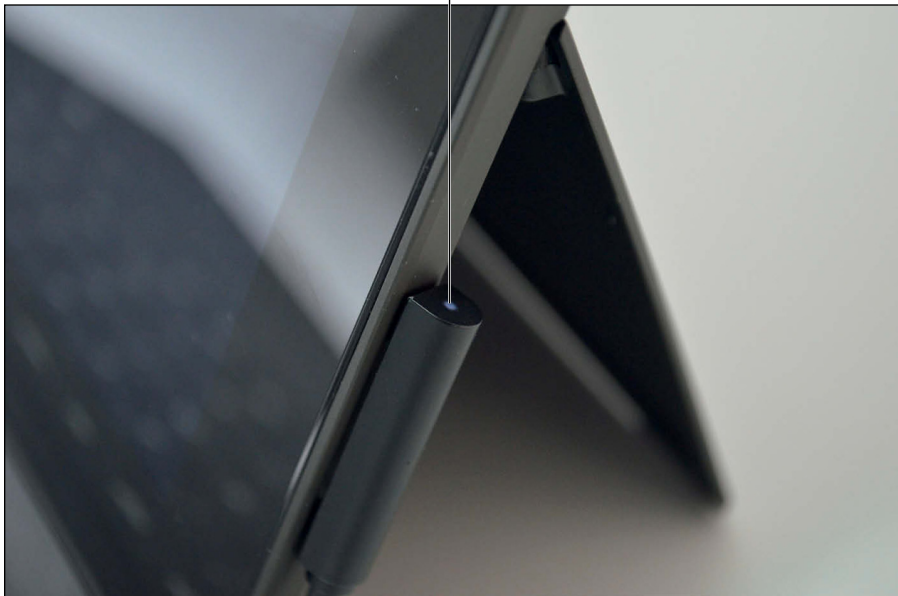
Figure 2-4: When the connector's light glows, you've successfully fastened it, and the Surface begins charging.
