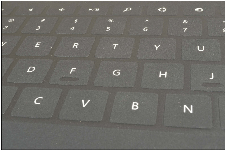
Figure 5-1: The Surface Touch Cover and Touch Cover 2 keyboards don't move when touched.
