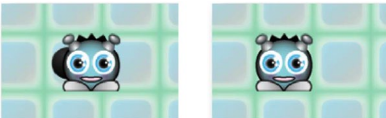
Figure 3-12. Detect a collision only when every corner point is inside the map cell
