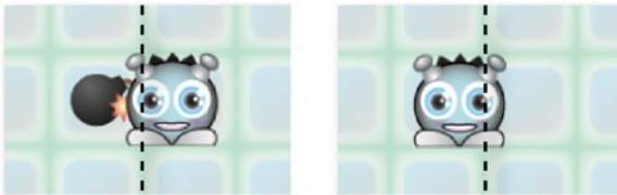
Figure 3-9. The sprite's center point is used to figure out its map location
