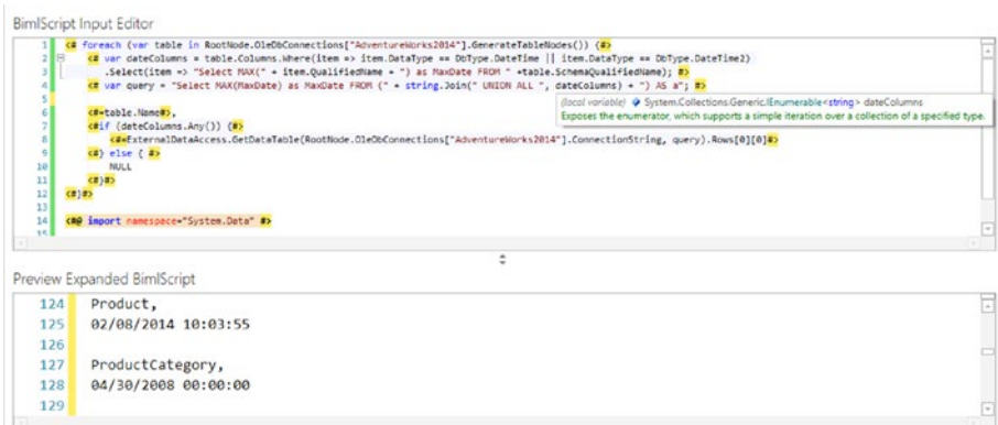
Figure 12-7. Generating profile statements with the same code from Listing 12-13 but in C#
