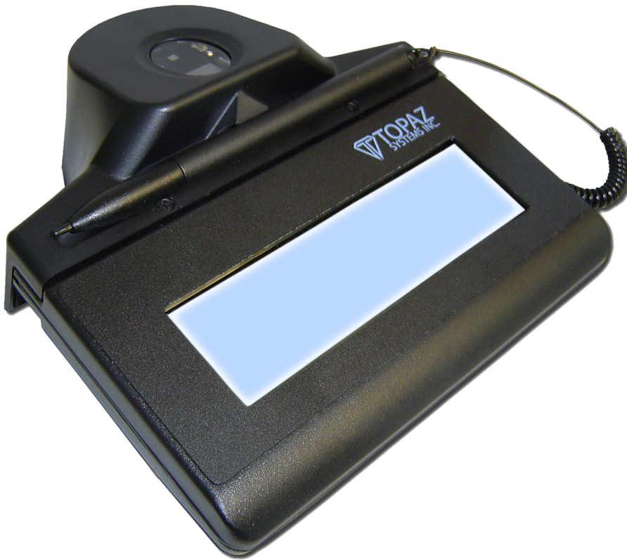
FIGURE 1.14 A fingerprint reader scans the loops, whorls, and other characteristics of a fingerprint and compares it with stored templates. When a match is found, access is granted. PHOTO OF BIOMETRIC ID SIGNATURE PAD WITH OPTICAL FINGERPRINT SENSOR (MODEL TF-LBK464) COURTESY OF TOPAZ SYSTEMS.
