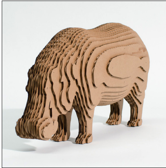
FIGURE 19-4: A typical cardboard model of a hippo made from slices that have been laser cut using an SVG file per slice.
