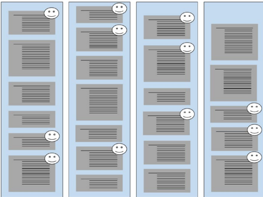
Figure 11-2. Depiction of the four thread dumps taken earlier, one tall blue rectangle per thread dump. Each gray box is a single stack trace, aka thread. The smiley faces point to the only stack traces executing code in the com.github.eostermueller package space.
