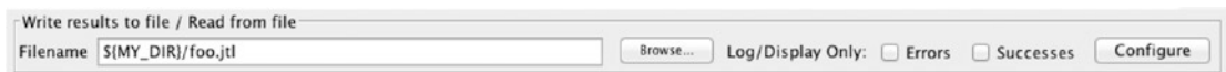
Figure 7-10. After restarting JMeter, if you want to reload metrics into a graph from a populated .jtl file, make sure the .jtl file name is specified, set UI focus in this text box, and press Enter
