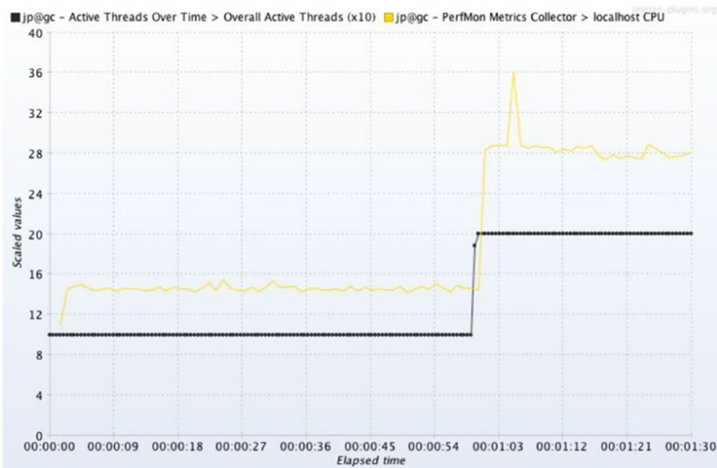
Figure 6-3. Discovering how many threads it takes to push the CPU to 25%. This graph with two different metrics (CPU and active threads) was made possible by Composite Graph and PerfMon, both from jmeter-plugins.org . Learn how to use them in Chapter 7 on JMeter.
