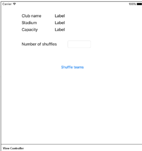
Figure 2-4. The iOS user interface. It has been designed using the universal class setting to ensure it works on all sizes of iPhone. The app has been set to be iPhone/iPad rather than universal.
