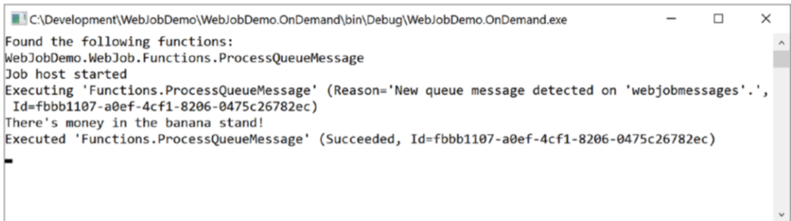
Figure 8-11. The WebJob console shows that our message was picked up, processed, and dequeued
