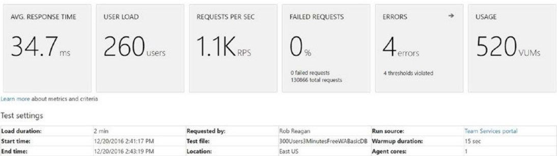
Figure 2-14. Results for the first load test
