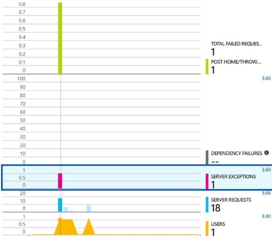
Figure 11-17. The Failed Requests time series charts give details on how many requests failed, whether the failure was due to a dependency (like a database) or a server exception, and how many users were affected
