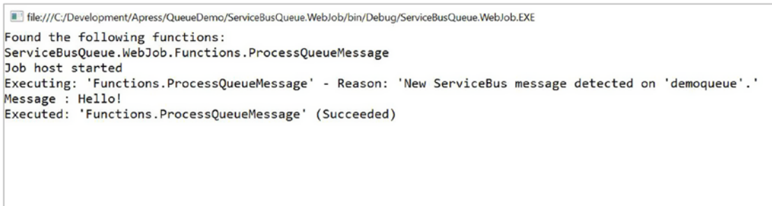
Figure 9-15. Our WebJob's console window after starting up and receiving a message from our Service Bus queue
