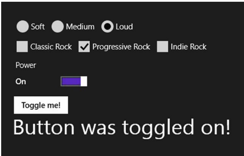
Figure 3-18. Radio buttons, check boxes, a toggle switch, and a toggle button
