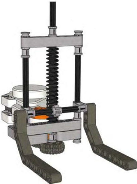
Figure 9-10. In this forklift-type powered attachment, as the worm gears turn, the forks will raise or lower depending on the motor's direction
