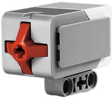
Figure 1-8. An EV3 Touch Sensor
