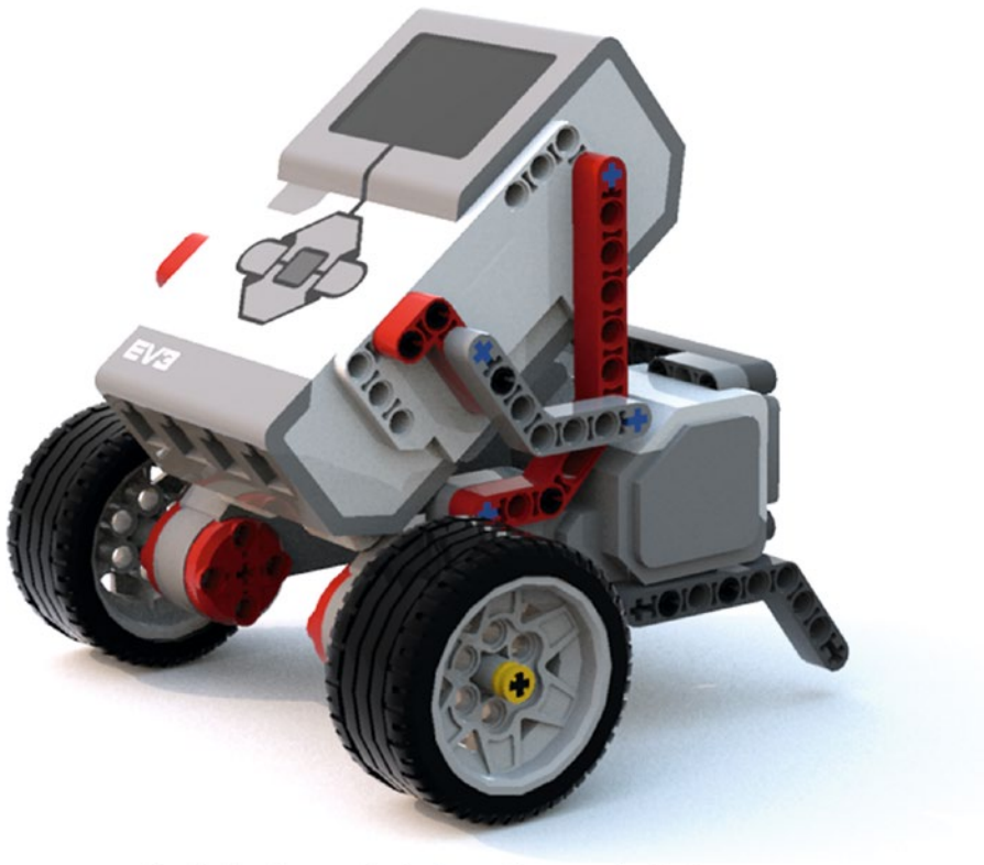
Figure 2-20. A two-wheeled robot with skids in the rear for balance
