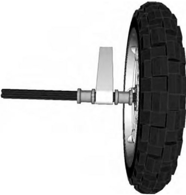
Figure 2-17. Single bushing spacing on wheel axle
