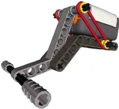
Figure 7-8. A release state bumper that, when pushed, releases the Touch Sensor instead of pressing it
