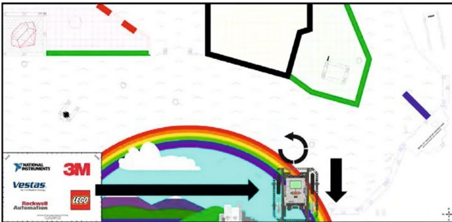
Figure 6-5. The path on the FIRST LEGO League 2008 Climate Connections mat that the robot follows as it follows the code in Figure 6-4: After making the 90-degree turn, the robot backs up and squares with the wall
