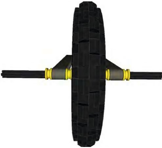
Figure 3-4. With the axle and wheel supported evenly on both ends, the friction is reduced drastically, and you get a much more stable drive system for the robot
