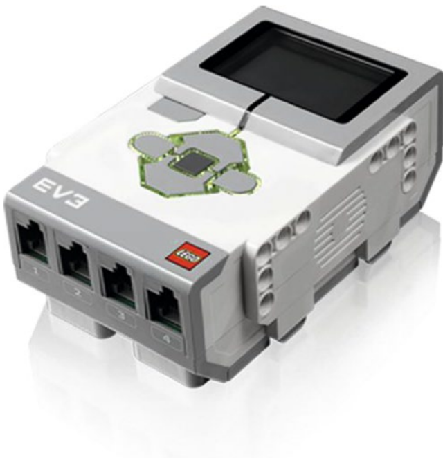
Figure 1-7. EV3 intelligent brick
