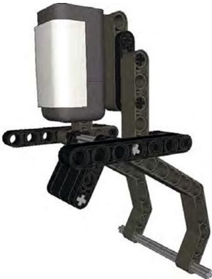
Figure 7-12. With the bumper pushed the black beams are removed from the view of the Color Sensor
