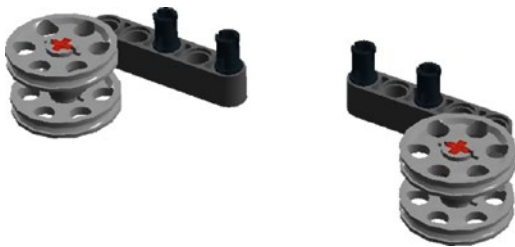
Figure 3-12. A pair of simple wall follower wheels used on my DemoBot
