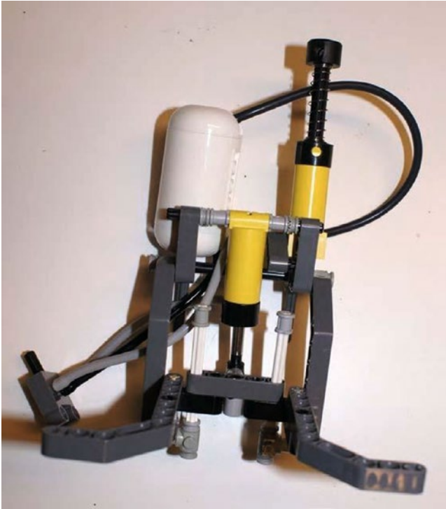
Figure 10-11. A robot's lifting attachment using pneumatics
