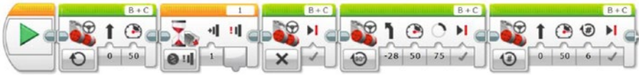
Figure 7-1. A simple EV3 program that drives forward until the Touch Sensor is pressed and then stops and turns
