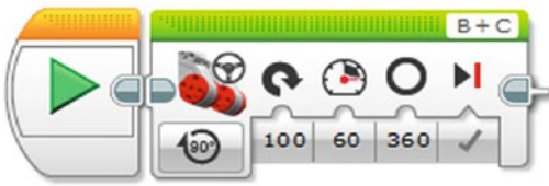
Figure 4-4. A Move Steering block being set to pivot the DemoBot 180 degrees by using the value of 360 as the degrees and the steering set to the far right
