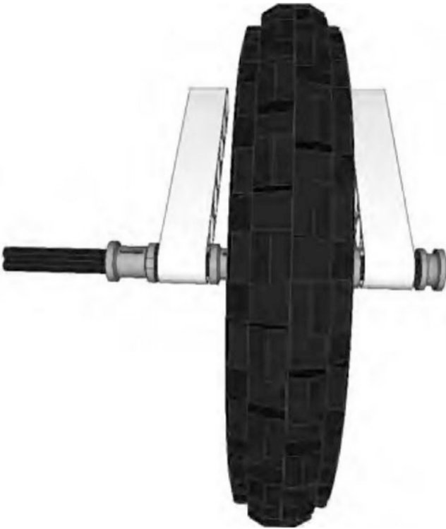
Figure 2-19. A wheel axle being supported on both ends, reducing friction on the axle
