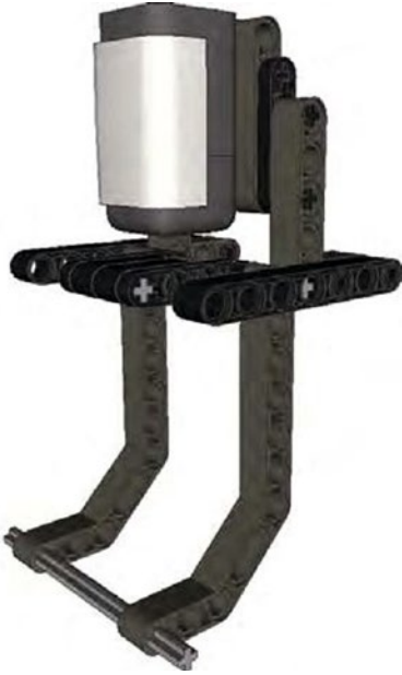
Figure 7-11. A Color Sensor being used to detect touch by a bumper that blocks the Color Sensor's path with black beams
