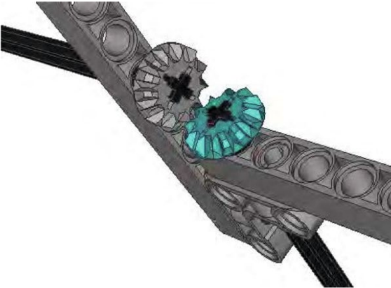
Figure 2-6. Bevel gears work well in tight areas but can only be paried up with other bevel gears
