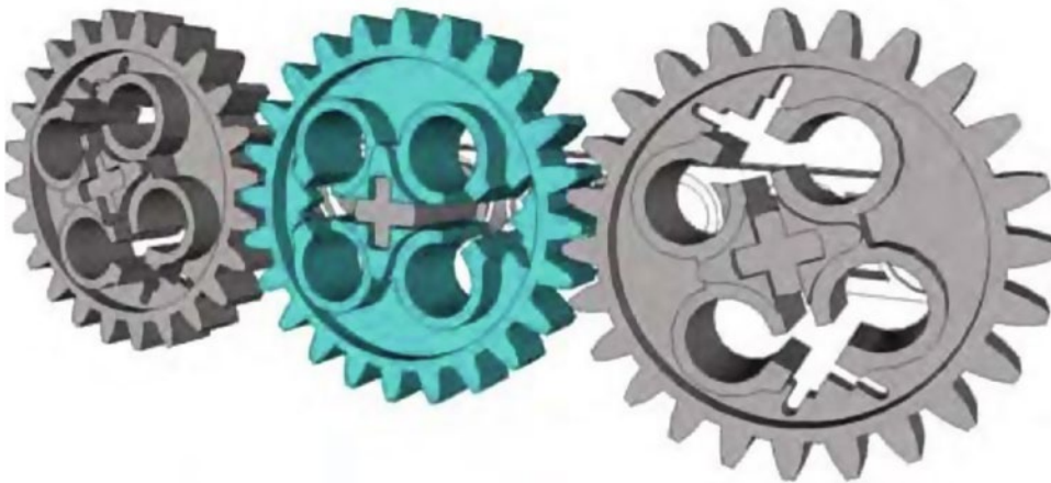
Figure 2-4. 24-tooth spur gears in line together
