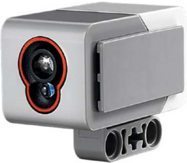
Figure 1-10. An EV3 Light Sensor
