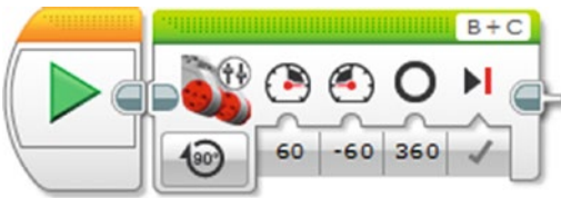
Figure 4-5. The Move Tank block being set to pivot the DemoBot 180 degrees by using the value of 360 as the degrees and setting the two motors in opposite directions
