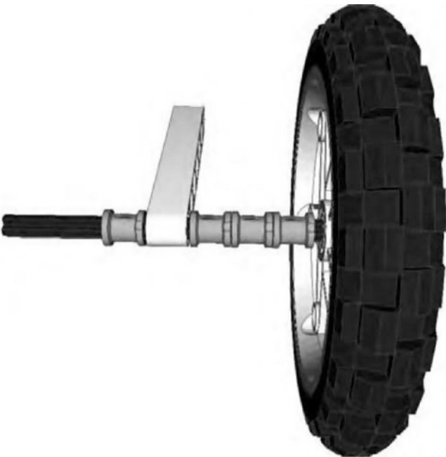
Figure 2-18. Multiple bushing spacing on a wheel axle, moving the wheel farther from the chassis and causing more friction
