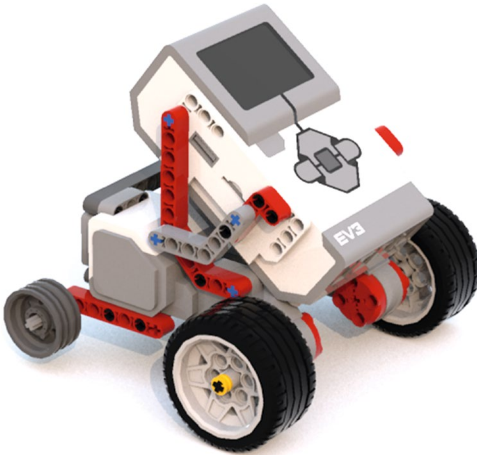
Figure 2-22. A four-wheeled robot with two-wheel drive
