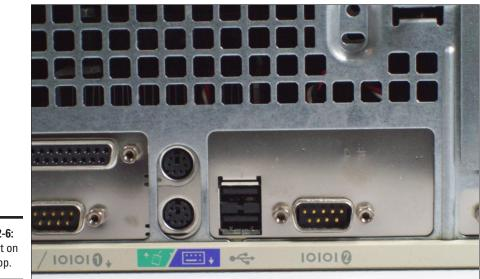
Figure 2-6: USB slot on a desktop.
