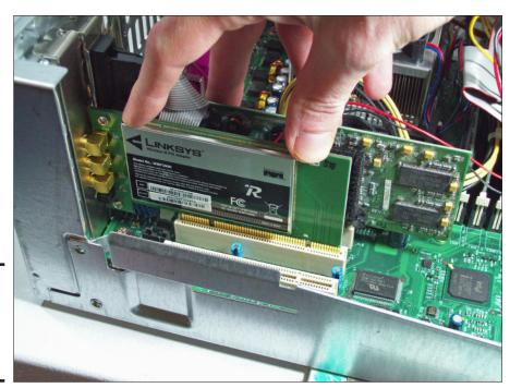
Figure 5-14: A PCI network adapter ready to be seated.
