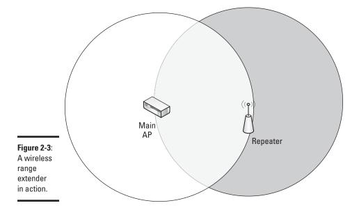
Wireless range extenders are the easiest way to get what you want, even though they're not the most efficient way about going about it. As you can see from Figure 2-3, the range extender has to be inside the coverage area of the main access point (white circle). This scenario has a fair bit of overlap between the two radios: a large part of the extended coverage area (dark circle) is already covered by the main access point.
