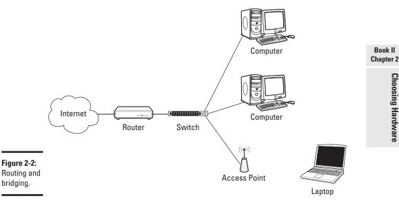
The router is routing between the stuff on the left and the stuff on the right. The network on the right is made up of the switch, the access point, and all the computers. The switch and the access point bridge all their connections to each other, which is how a small network grows.
