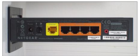
Figure 2-5: Switch ports on the back of your router.
