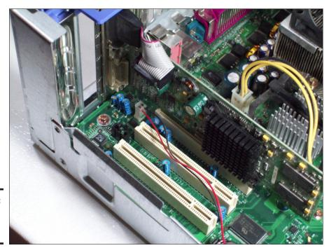
Figure 5-13: PCI slots in a standard desktop.
