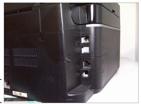
Figure 7-1: The wired port on the printer.
