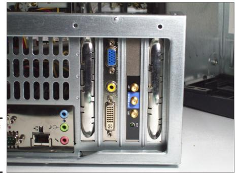
**Figure 5-15:** Antenna connectors on the wireless card.
