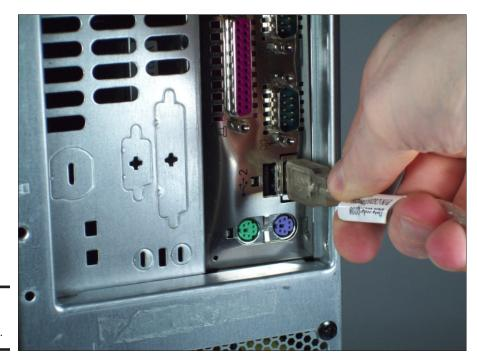
Figure 5-6: Plug in the USB cable.
