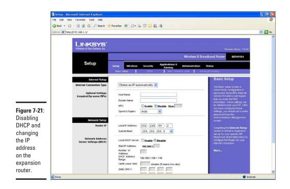
You might also note that the Internet connection stays on Obtain an IP automatically. This setting doesn't really matter anymore because the expansion router won't be plugged into the Internet.
