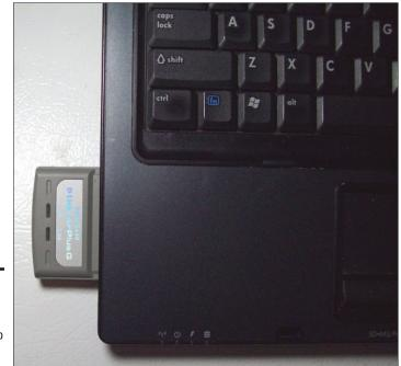
Figure 5-8: A PC Card that's been inserted into a laptop.
