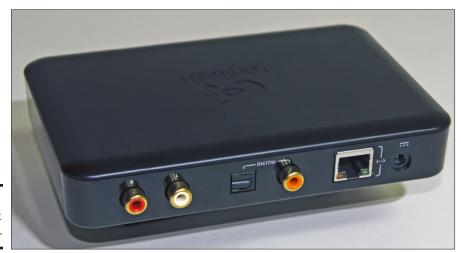
Figure 2-2: Squeezebox connections.
