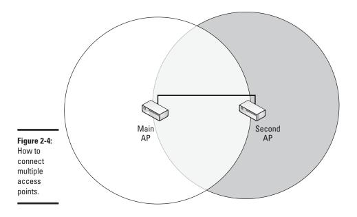
This option reduces the overlap between the two wireless zones because the two access points don't have to *see* each other over the wireless network. However, the two access points must somehow be connected over the wired network. Given that the benefit of wireless is avoiding wires, this option is cumbersome to set up. Figure 2-4 does show some overlap between the two access points, so that there is no dead zone between the two.
