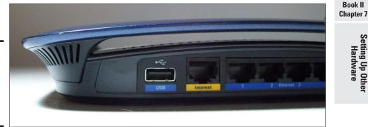
Figure 7-8: A USB port on a router for an external storage device.
