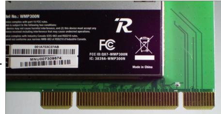
Figure 5-12: The edge connectors on a wireless card.
