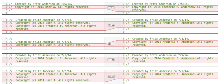
Figure 7.15 (top) When part of a file has picked up independent edits since the last common revision, it's a conflict, which Xcode highlights in red. Because it can't choose between them, the marker in the middle of the highlight ribbon contains a question mark. The control at the bottom of the Merge sheet lets you choose among (second through last) local-before-remote, local, remote, and remote-before-local.
