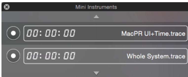
Figure 26.5 The Mini Instruments floating window. It lists each open trace document next to a clock and a recording button. Scroll through the list using the arrowheads at top and bottom.
