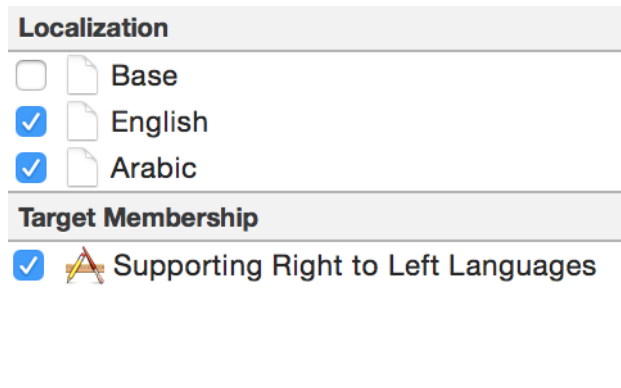
Figure 8-38. Localize the strings file so that you have both English and Arabic in the list
