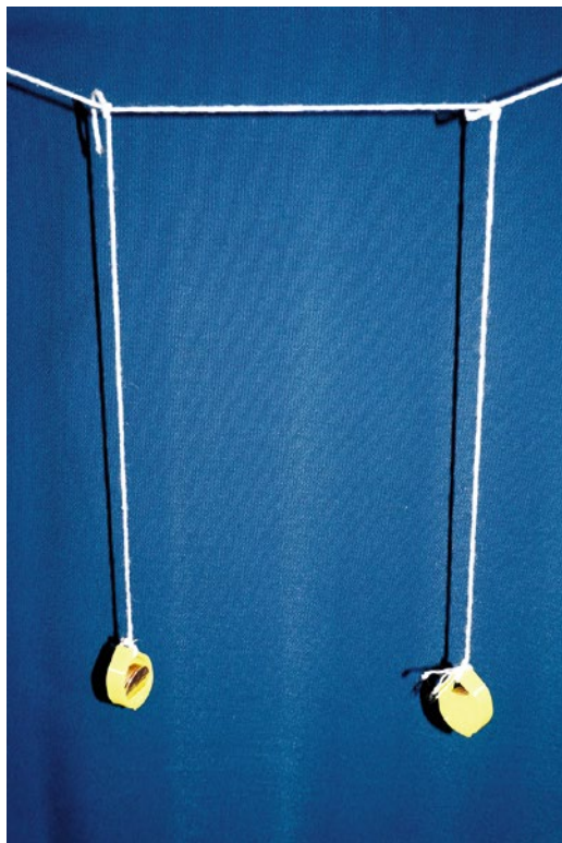
Figure 1-3. Coupled pendulum setup. Pendulums are free to swing toward and away from the camera during the experiment. Cloth was placed behind them to make them more visible for photograph.
