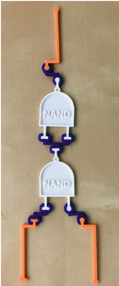
Figure 7-6. AND gate made up of NANDs (inputs on bottom, output on top)
