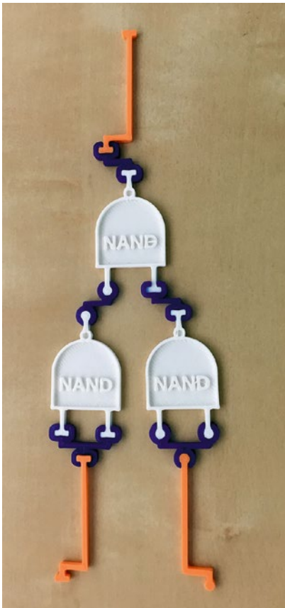
Figure 7-7. OR gate made up of NANDs (inputs on bottom, output on top)
