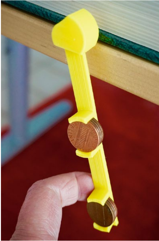
Figure 1-5. The experimental setup for the compound pendulum
