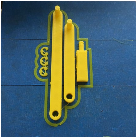
Figure 1-6. Double pendulum as printed. Stringing inside the snap rings needs to be removed.
