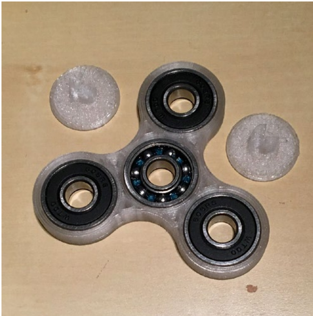
Figure 5-5. Fidget spinner: 3D printed parts plus roller skate bearings
