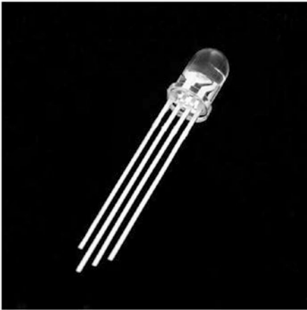
Figure 3-8. RGB LED with common anode form
