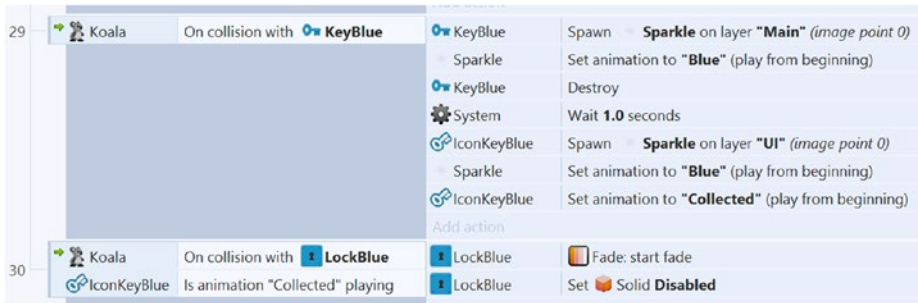
Figure 13-17. Events related to the key and lock mechanic
