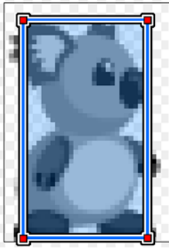
Figure 13-3. Collision polygon for the Koala sprite
