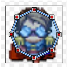
Figure 14-5. Collision polygon for the Hero sprite
