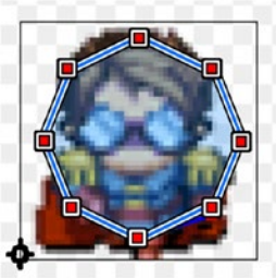
Figure 12-3. The Player sprite's circular collision polygon
