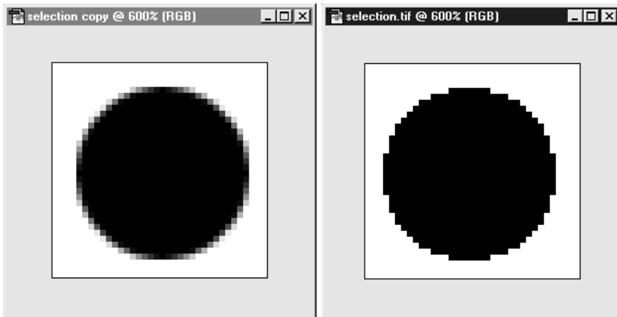
FIGURE 4-6 An anti-aliased elliptical selection on the left, and an elliptical selection without anti-aliasing on the right.
