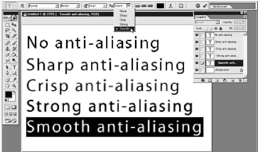
FIGURE 7-3 Choosing an Anti-aliasing setting may improve the text quality dependent upon the text's font and size.
