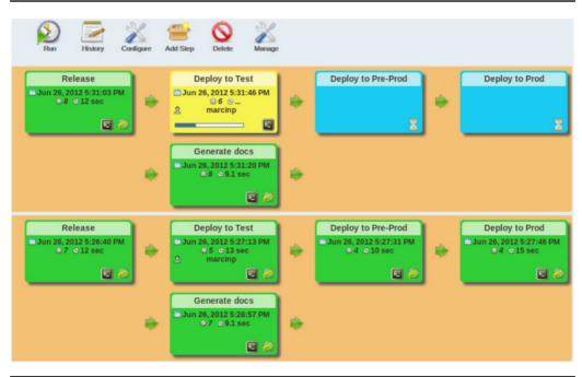
FIGURE 4-13. Graphical representation of a build pipeline
