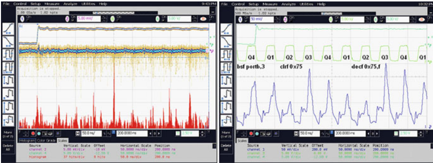
Fig. 7.8 Photon emission analysis and power analysis results for PIC16F628 microcontroller
