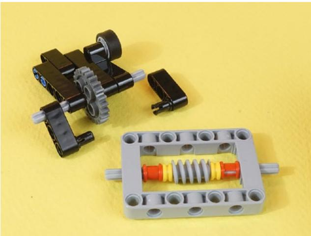
**Figure 11-22.** Side fasteners preparing to attach the Gear Yoke to the Worm Gear sub-assembly
