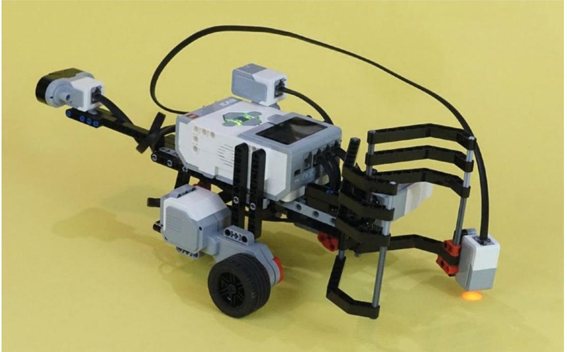
**Figure B-2.** The PushBot after being tested and hardware-validated with the Robot Commander app
