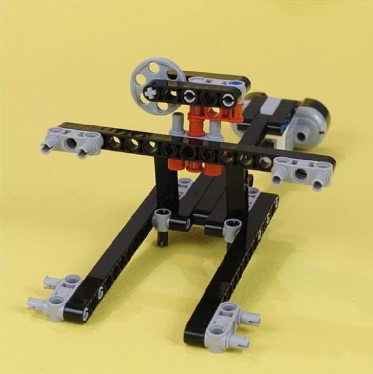
**Figure 19-48.** Turn it around to see the back side of the Neck/Infrared Sensor•caster wheel and frames
