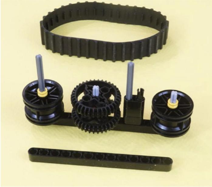
**Figure 15-8.** The second hub and the gear-wheel assembly are in place. The remaining 13-hole beam is ready to be mounted. The single black pin in the center will keep the beam from falling off. Mount the beam so all three axles go through. Then stretch the tank-tread over the end hubs.
