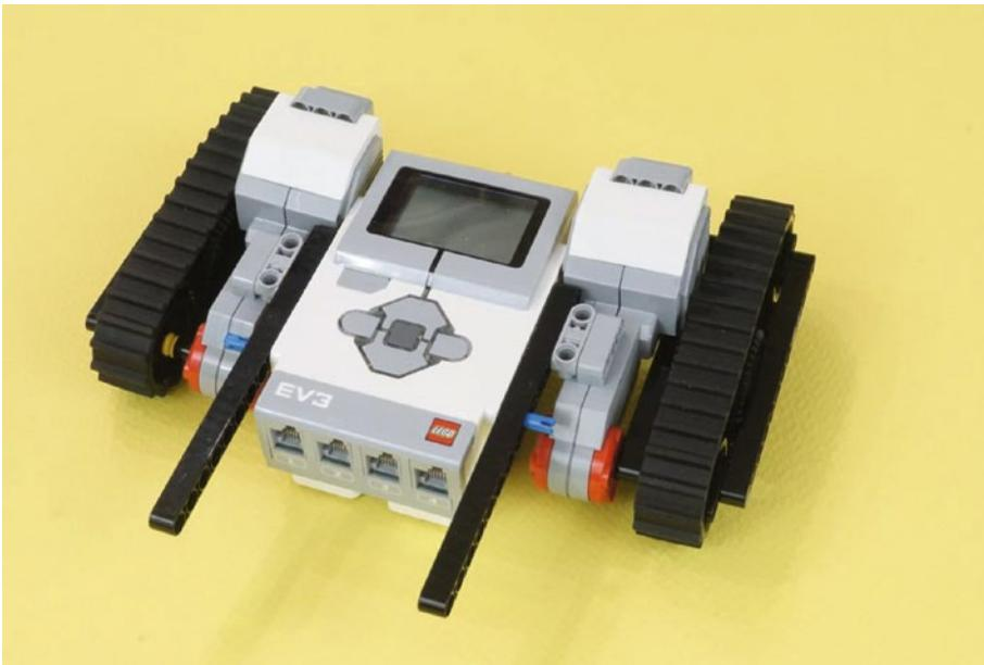
**Figure 15-15.** Both tank-tread motor assemblies in position
