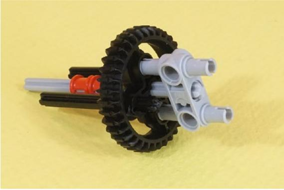
**Figure 7-21.** The double gray connector about to be fully inserted in the third gear. See [Figure 7-23](#) for a side view of this part.
