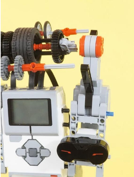
**Figure 7-44.** *The right-side motor clips on to your StringBot*
