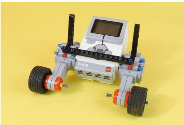
**Figure 11-8.** The basic body, with hardpoints
