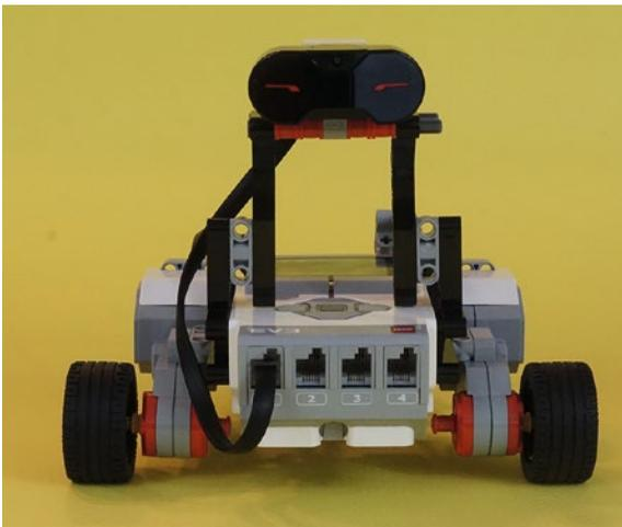
**Figure 3-35.** The Infrared Sensor connects to port 1
