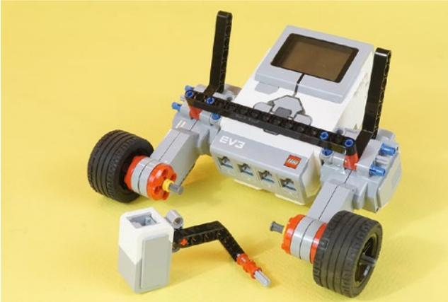
**Figure 11-10.** *The Color Sensor assembly*
