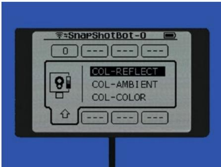
**Figure 10-7.** *Selecting the COL-REFLECT mode*
