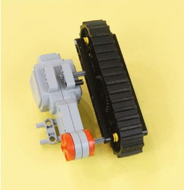
**Figure 15-11.** Insert the lower axle into the motor and the upper axle into the axle socket in the motor mount. Connect the double gray component to the other side. The second motor will be a mirror image of this.
