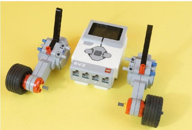
*Figure 11-4. Both sides assembled, ready to be fastened to the Brick*
