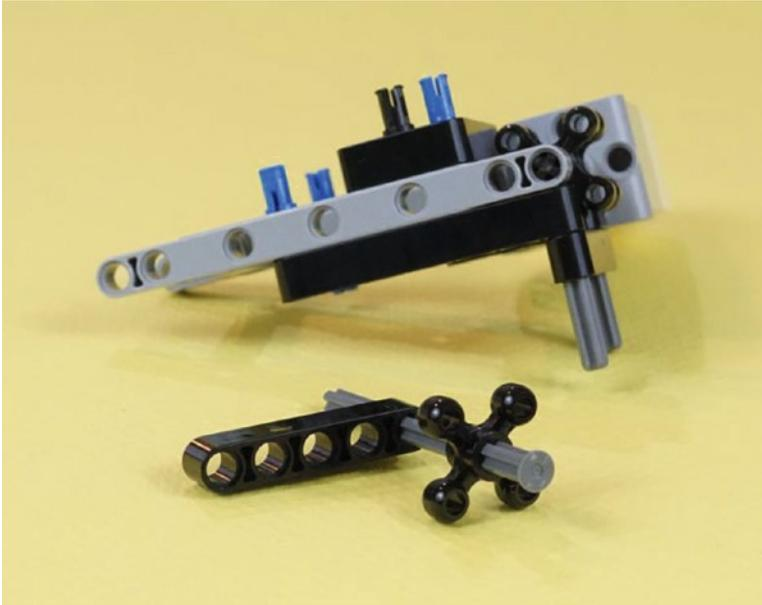
**Figure 19-9.** The corner of the large L-beam engages the blue pin as shown. The black pin goes in just to the left of the blue pin. The long side of the L-beam points away from you. The three-hole short side is directly facing you. Pressing this sub-assembly down gets you to Figure 19-10.
