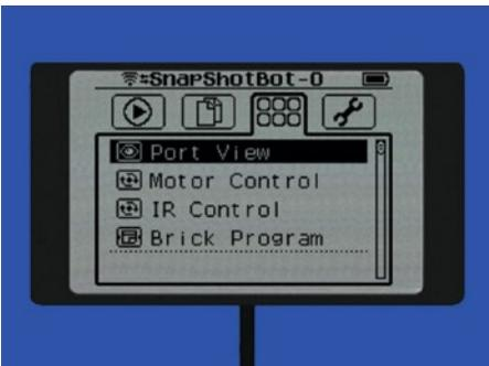
**Figure 10-5.** The View screen with the Port View selection highlighted
