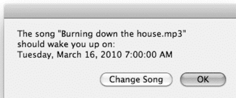
Figure 9–6. The script displays a dialog box that allows the user to change the song. The dialog box will give up (close by itself) after 15 seconds.
