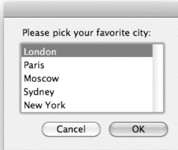
Figure 16–17. The dialog box resulting from the choose from list command with the default items parameter
