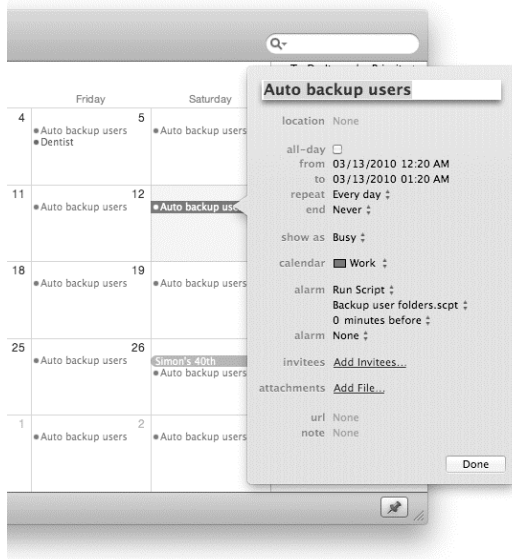
Figure 23-4. The event shown will run the Backup user folders.sct script every night at 12:20 AM.
