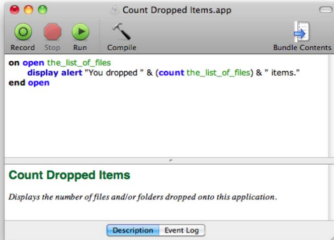
Figure 4–15. You can add formatted text to the Description panel in the AppleScript Editor script window. This text can be displayed when the script applet starts.
