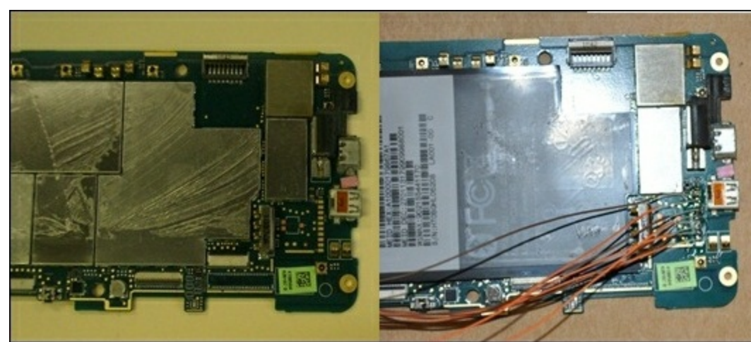
HTC Evo before and after being hooked up for JTAG (courtesy of http://lowcostwin4n6.blogspot.com/ )
