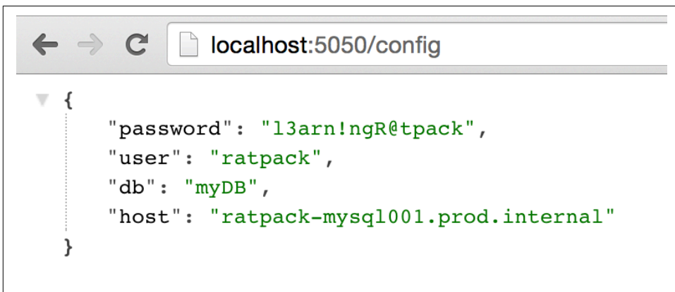
Figure 4-3. Configuration JSON with environment config
