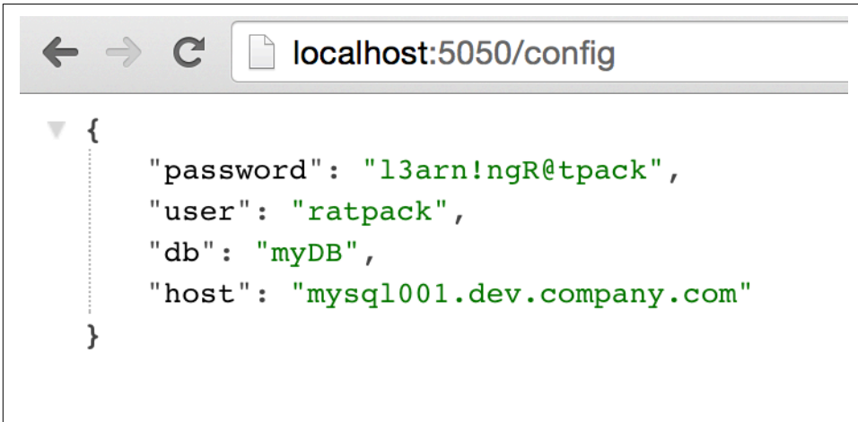
Figure 4-2. Configured DatabaseConfig JSON
