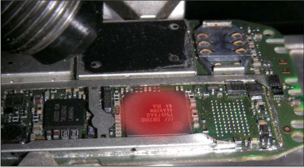
The preceding image shows a device's chip about to be removed (source: [https://pressdispensary.co.uk/image\\_library/q991448.html](https://pressdispensary.co.uk/image_library/q991448.html)). Once the chip is successfully removed, the examiner must prepare adequate memory-reading hardware, a chip adapter, and the software that goes with it. Depending on the chip's nature (**Thin Small Outline Package (TSOP)** type, or **Bag Grid Array (BGA)** type), the cost of handling it varies.
