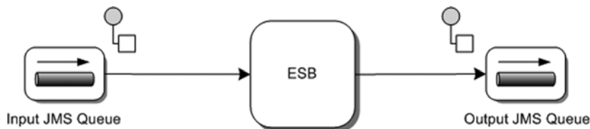
Figure 6.2 This JMS example shows how to use the ESB to consume a message from a JMS queue and produce the message for another JMS queue.
