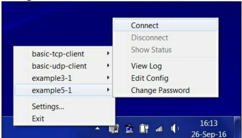
9. Verify that the VPN connection is established and that the log file, c:\temp\openvpn.log, has been created.
