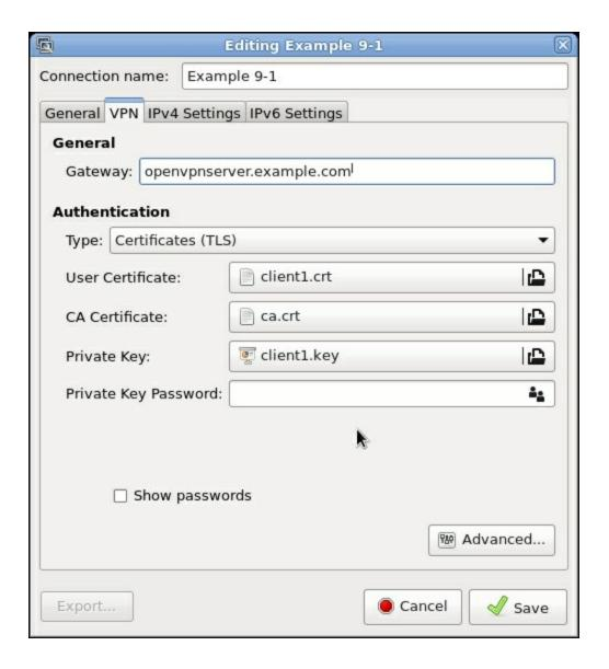
The **Type** of authentication is **Certificates** (**TLS**). Then, for the **User Certificate**, **CA Certificate**, and **Private Key** fields, browse to the directory where the client files client1.crt, ca.crt, and client1.key are located, respectively. Fill in the **Private Key Password** fields, if required. Do not click on the **Save** button just yet, click on **Advanced...** instead.
