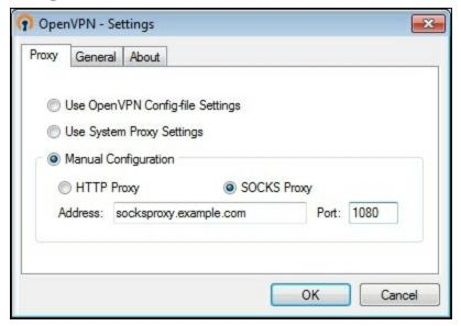
3. Set up a **SOCKS proxy** by setting up an SSH connection on the intermediary proxy host. The destination address for the SSH connection is a server which can reach the OpenVPN server:
