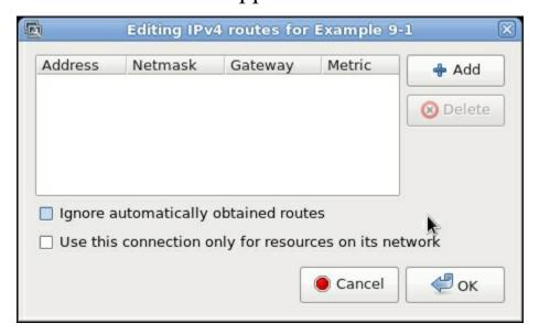
Routes pushed by the server can be overruled using the **Ignore** automatically obtained routes option. By default, the <code>NetworkManager-openvpn</code> plugin will enable <code>redirect-gateway</code>, even if it is not pushed by the server. This behavior can be overruled by checking the **Use this** connection only for resources on its network checkbox.
