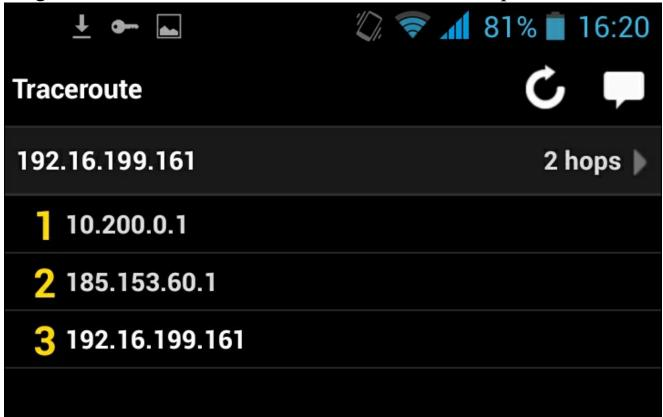
6. The first address in the traceroute output is 10.200.0.1, demonstrating that the traffic is redirected via the OpenVPN server.
