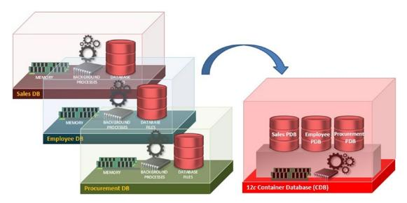
Figure 10-2. Oracle Database multitenant architecture
