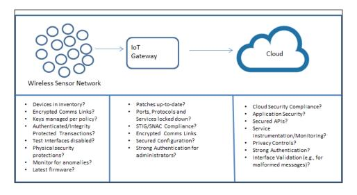
We can evaluate collected security-relevant data by considering an IoT architectural model of WSN endpoints transmitting data to a protocol gateway, then that gateway passing the data to the cloud. Once in the cloud, we can leverage the capabilities of the **cloud service provider (CSP)** to capture data between application endpoints supporting the IoT sensors. For example, within Amazon we can leverage AWS CloudTrail to monitor API calls to the cloud.
