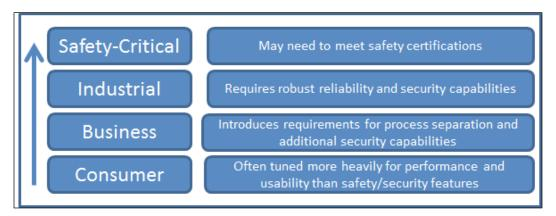
At the top end of the spectrum (safety-critical IoT devices), RTOS selection should be based heavily on whether there is a need to meet industry-specific standards. Examples of these include the following:
