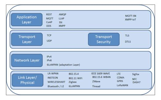
This figure provides a view into some of the better-known protocols that can be implemented by IoT devices to form a complete communications stack.
