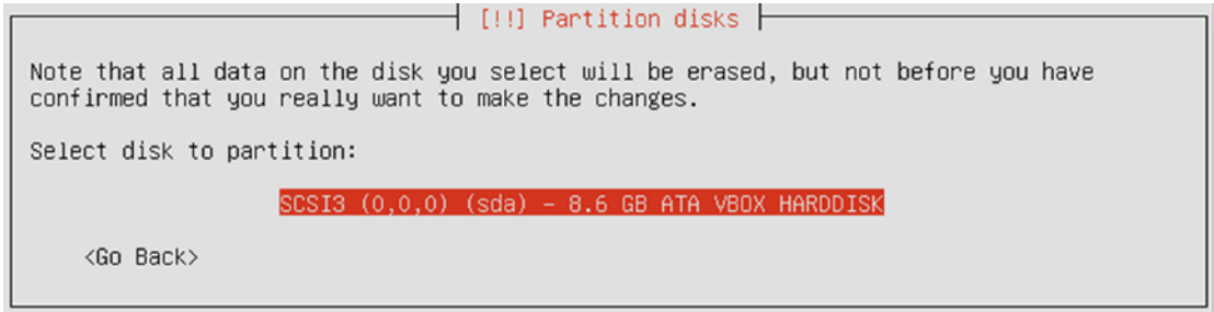
Figure 2-55. Choosing the disk to partition
