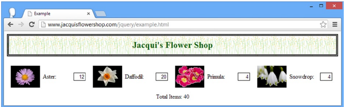
Figure 14-6. The effect of processing the data returned from the Ajax POST request
