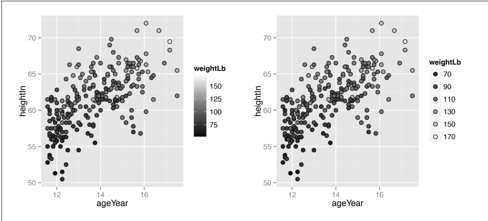
Figure 5-10. Left: outlined points with a continuous variable mapped to fill; right: with a discrete legend instead of continuous colorbar
