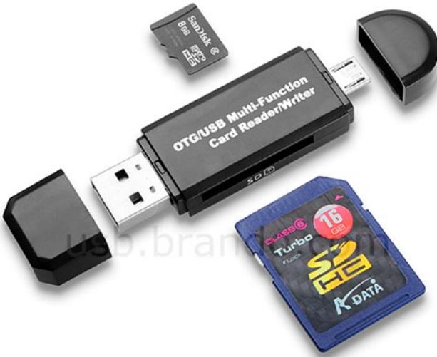
**Figure 1-5.** Card reader and microSD-to-SD adapter
