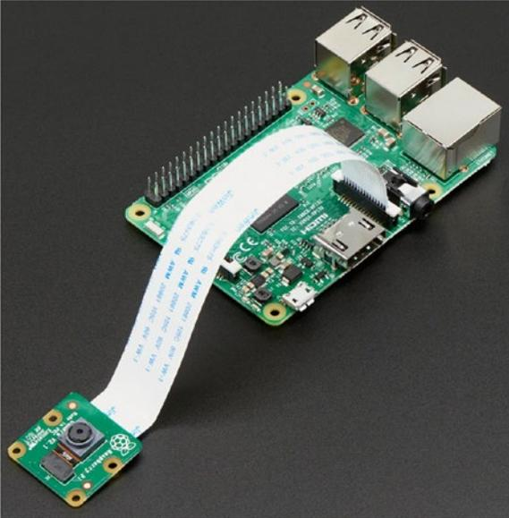
**Figure 3-4.** Attaching the Pi Camera module to the Pi
