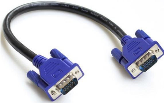
**Figure 1-7.** VGA male-to-male cable (also known as a D-SUB cable)
