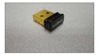
You'll also need to connect a powered USB hub for this process so that you can access the wireless keyboard, as well as the USB wireless LAN device. Now, connect the hub to the Raspberry Pi, and then connect your keyboard and the device to the powered hub.
