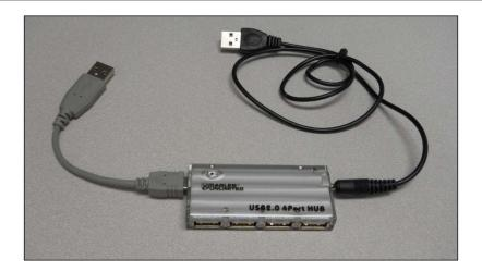
Notice that on this hub, there are two connections. The one to the far right is a power connection, and it will be plugged into a battery with a USB port. The connection to the left is the USB connection, which will be plugged into the Raspberry Pi.
