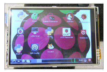
You can also purchase a display unit with HDMI input; here is one that is available from www.adafruit.com, connected to Raspberry Pi B+:
