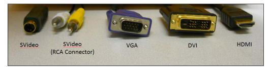
There is an HDMI connector on the Raspberry Pi A+ and B+. To use this connector, simply connect your cable with regular HDMI connections to Raspberry Pi and your TV or monitor that has an HDMI input connector. HDMI monitors are relatively new, but if you have a monitor that has a DVI input, you can buy relatively inexpensive adapters that provide an interface between DVI and HDMI.
