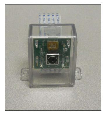
The camera connects to the Raspberry Pi by installing it into the connector marked camera on the Raspberry Pi. To see how this is to be done, see the video at http://www.raspberrypi.org/help/camera-module-setup/.
