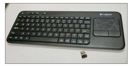
This is a Logitech keyboard. Logitech generally makes very reliable keyboards and these connect well to Raspberry Pi. This keyboard is available online on Amazon and at most electronics or computer stores. You'll notice that this version has a built-in mouse pad.
