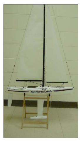
In fact, many RC-controlled boats can be modified to use Raspberry Pi. All you need is space to put the processor, the battery, and any additional control circuitry. In this case, the sailing platform has two controls, a rudder, which is controlled by a servo, and a second servo, which controls the position of the sail, as shown in the following image:
