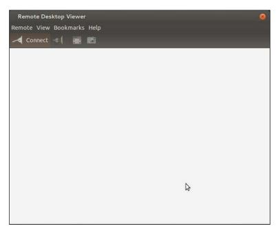
Make sure vncserver is running on the Raspberry Pi. The easiest way to do this is to log in using SSH and run vncserver at the prompt. Now, click on **Connect** on the **Remote Desktop Viewer**. Fill in the screen as follows; under the **Protocol** selection, choose **VNC**, and you should see the following screenshot:
