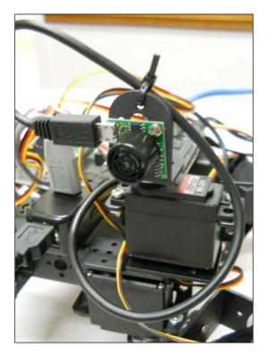
Make sure you connect your servo to the servo controller; it can fit into any open connection. I am connecting mine to my quadruped robot that has eight servos to control, so I have connected mine to the eighth connection on the servo controller board, as follows:
