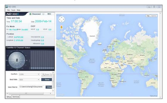
5. Unfortunately, if you are in a building or a place where receiving information from the GPS satellites is difficult, the device may struggle to find its position. If you want to find out whether or not the system is working, even though it may struggle to find the signals, select the **Terminal** tab selection in the lower-left corner of the screen. You should see what is shown in the following screenshot:
