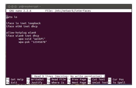
The wpa-ssid and wpa-psk values here must, of course, match what your wireless access point requires. Reboot, and your device should be connected to your wireless network.
