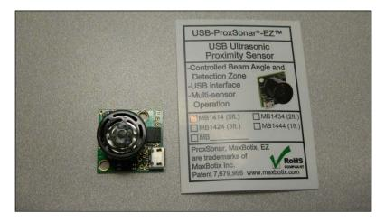
It is the USB-ProxSonar-EZ sensor, and can be purchased directly from MaxBotix or Amazon. There are several models, each with a different distance specification; however, they all work in the same way.
