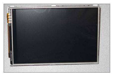
The unit simply plugs into the GPIO connector on the Raspberry Pi. Simply download the image from the page shown on Amazon, unzip the file, burn a card, and plug in the display, and you can get a simple display on your Raspberry Pi, as follows:
