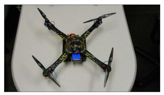
The quadcopter has two sets of counter-rotating propellers. This simply means that two of the propellers rotate one way, while the other two rotate the other way, to provide thrust in the same direction. This provides a platform that is inherently stable. Controlling the thrust on all four motors allows you to change the pitch, roll, and yaw of the device. The following figure may be helpful to understand this concept:
