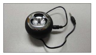
Fortunately, these devices are very inexpensive and widely available. Make sure the speaker is powered because your board will generally not be able to drive a passive speaker with enough power for your applications. The speaker can use either internal battery power, or can get its power from a USB connection.
