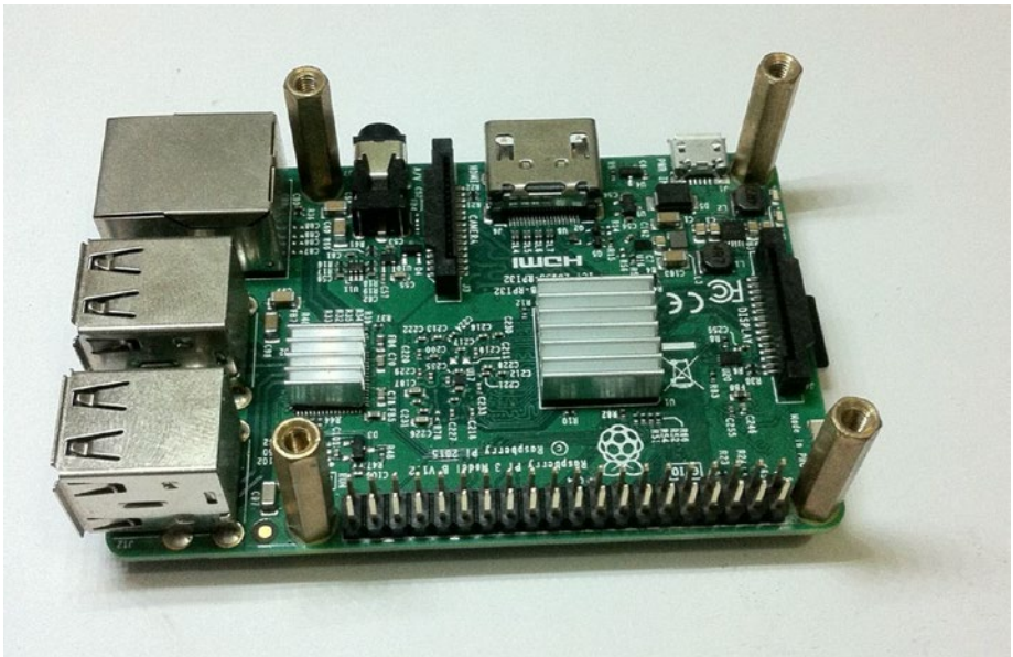
Figure 6-6. Attaching male-to-male standoffs to the Pi
