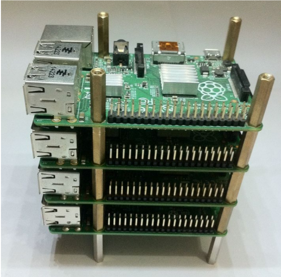
Figure 6-9. Raspberry Pi Supercomputer stack
