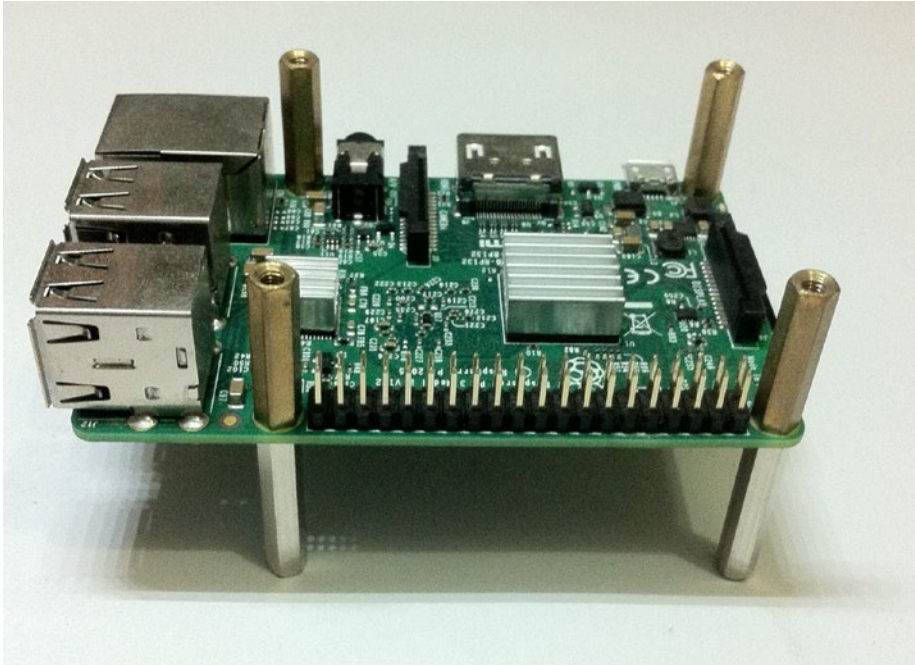
Figure 6-7. Attaching female-to-female standoffs to the cluster base
