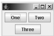
Figure 8-9. An example of FlowLayout when the container has been reduced in size
