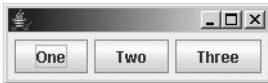
Figure 8-7. FlowLayout showing the default operation—all components laid out at their preferred size next to each other
