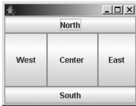
Figure 8-6. An example of the BorderLayout in action
