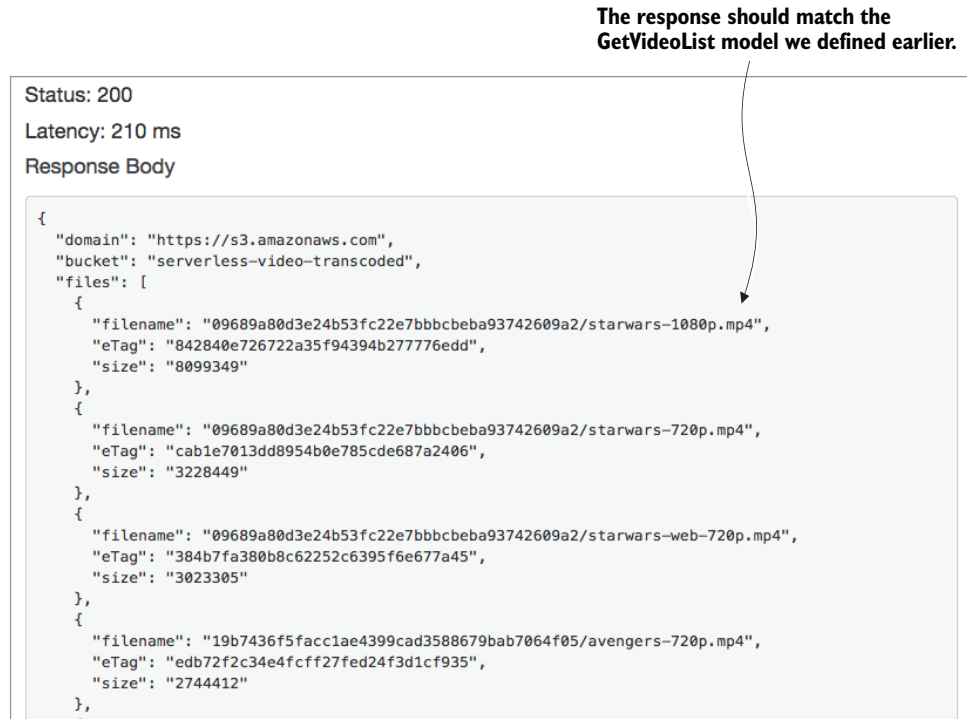
Figure E.6 The response from the API should be different when the new model is implemented.
