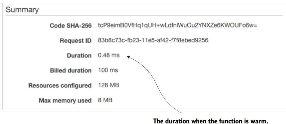
Figure 6.4 A warm function runs much quicker than a cold one.
