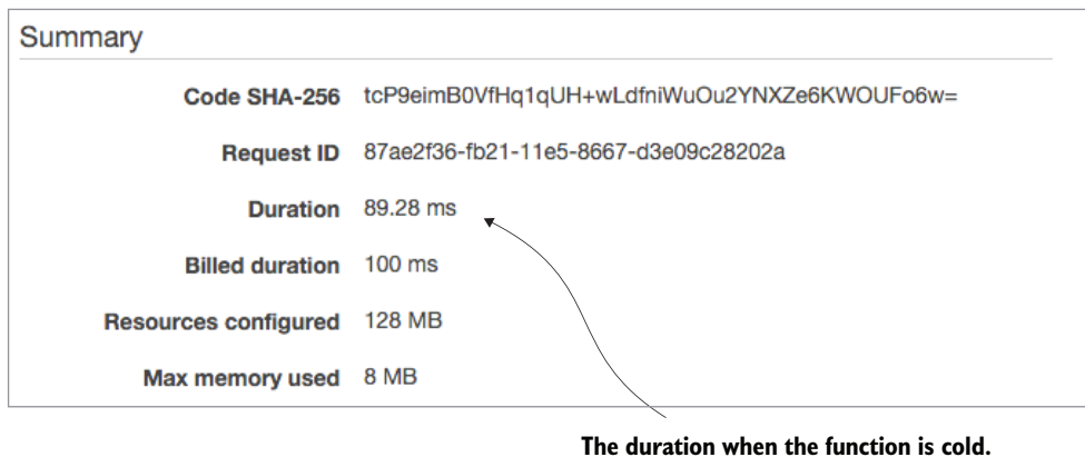
Figure 6.3 The time it takes to run a cold function is nearly 90 ms.
