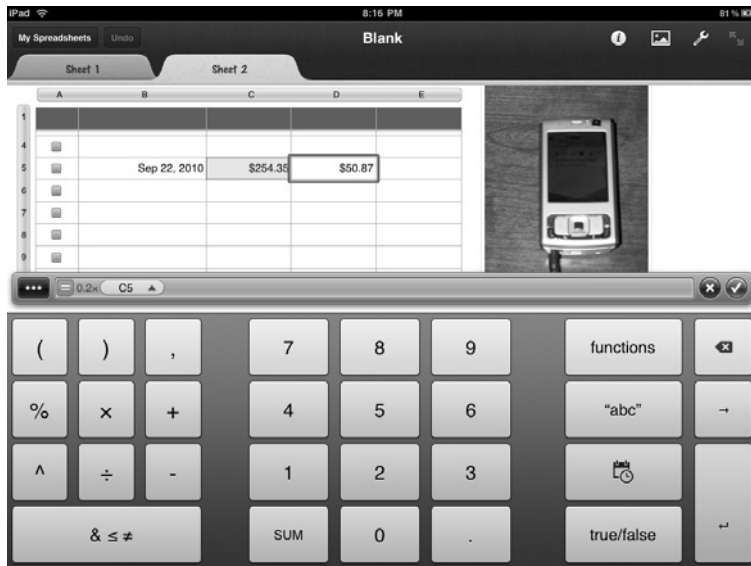
Figure 14-20. The formula entry keyboard is used to enter both simple and complex formulas into spreadsheet cells.
