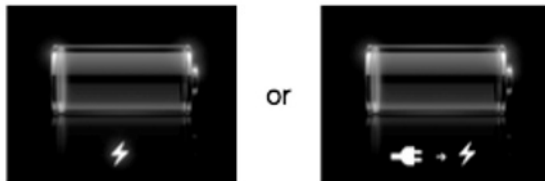
Figure 3-12. If you see either of these symbols on your iPad screen, stop using it, and plug it into a power source as soon as possible.
