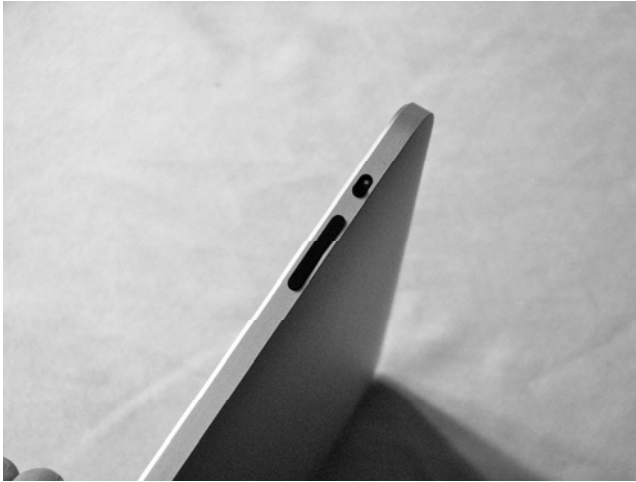
Figure 3-2. The screen rotation lock (the small switch) and the volume toggle (the larger button)
