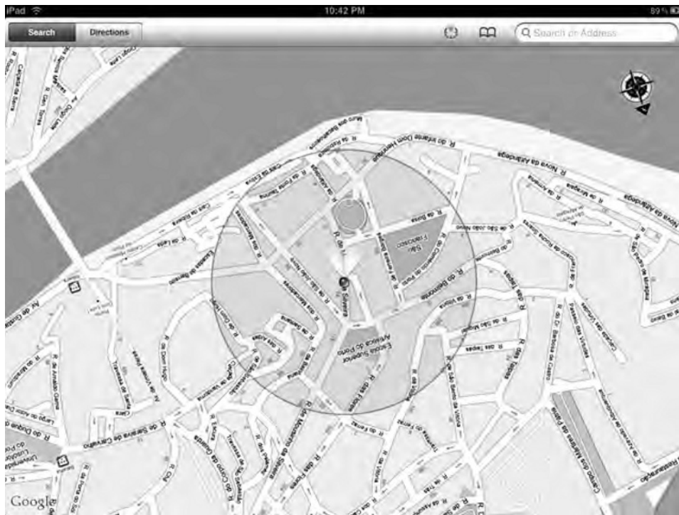
Figure 12-17. Digital Compass mode. This is the same image as in Figure 12-14 but with the Digital Compass turned on. Notice how the map is pointing the other direction? That's because the iPad is facing that direction, which in this case is south. Note the compass pointing north in the upper-right corner and the “headlight” emanating from the blue current location dot.
