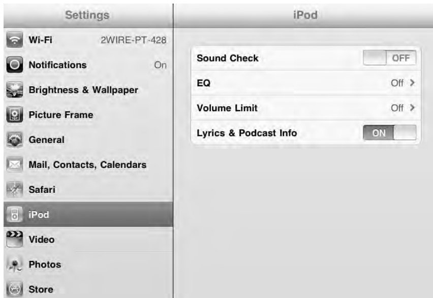
Figure 7-35. The iPod app's settings allow you to set EQ and adjust volume limits.
