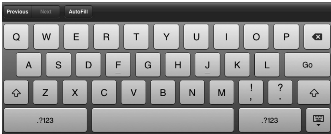
Figure 6-8. The text entry keyboard for web page forms. Notice the Previous, Next, and AutoFill buttons at the top.
