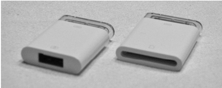
Figure 1-7. The iPad Camera Connection Kit includes two adapters. The one on the left connects to a standard USB cable for direct connection to a digital camera, while the adapter on the right can be used to read or write SD memory cards.
