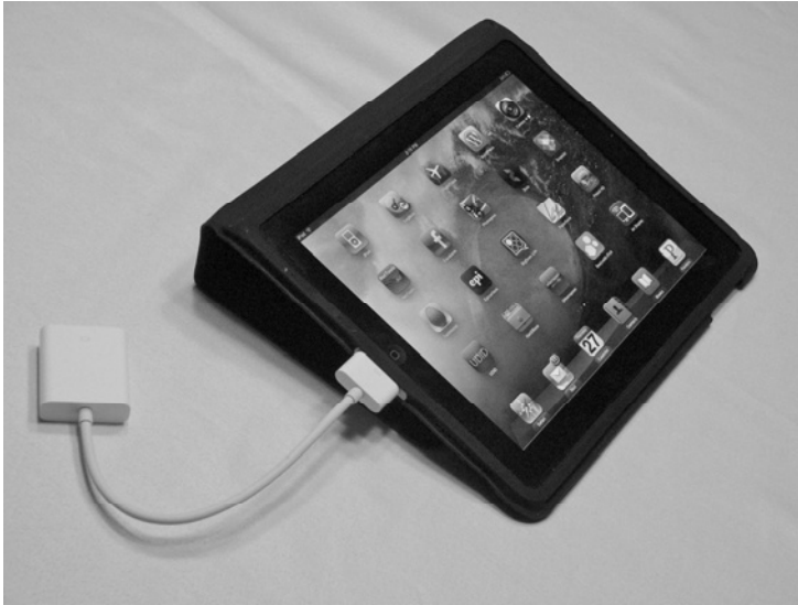
Figure 3-15. The iPad Dock Connector to VGA Adapter is useful for displaying Keynote presentations on an external monitor or PC projector.
