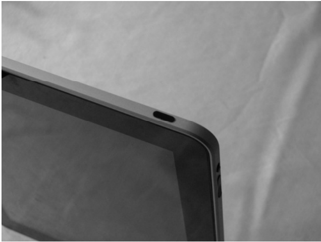
Figure 3-1. The Sleep/Wake button is used for powering the iPad on or off and for putting it to sleep when it's not being used.
