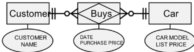
Figure 5-11. An associative entity should not be used to resolve a many-to-many relationship
