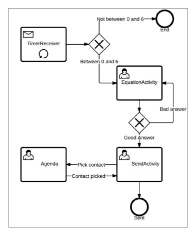
First of all, our broadcast receiver class named TimeReceiver will receive a time change message from the Android operating system every minute. If the time is between 12 a.m. and 6 a.m., the Equation activity will be launched. In this activity, we ask the user to solve a simple equation and launch SendActivity in case the correct answer is given. In SendActivity, we ask the user to pick a contact in their agenda and retrieve the picked contact. Finally, the user can write their SMS and send it.
