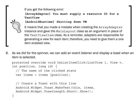
The previous code has to be added in the Main class and override the default OnListItemCLick() method of the ListActivity class. In this override, we receive the ListView, the view, the position of the selected item, and a unique id. We use the position of the clicked item to retrieve the state name in the item array and then create a simple Toast. The following screenshot shows the interface after a click:
