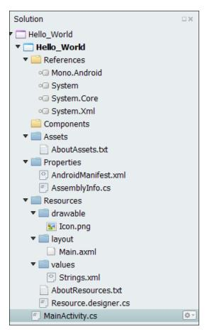
4. Open the Main.axml file in the Layout folder under Resources. A new file containing the graphical interface of your Hello World! app should appear.
